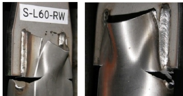
Fig. 5 Typical deformed shapes observed for CHS and SHS members with long weld lengths
