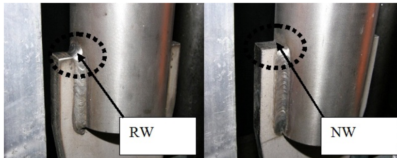
Fig. 3 View of the slot end conditions with / without a return weld
