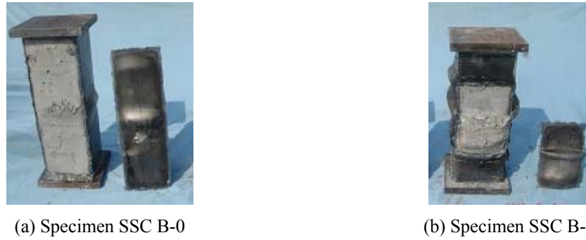
Fig. 9 Failure modes of the in-filled concrete
