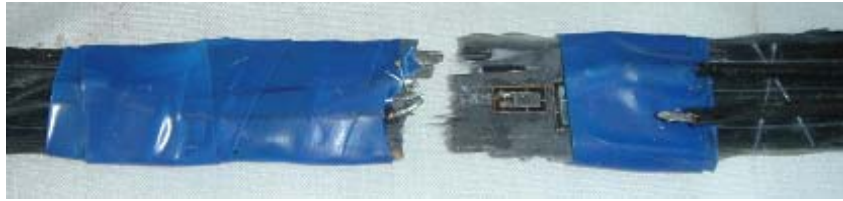
Fig. 3 Typical failed CFRP coupon
