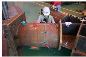
① Attachment of strain gauges
