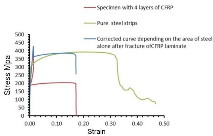
(a) Stress-strain curves of specimen with 4 layers of CFRP and pure steel strips
