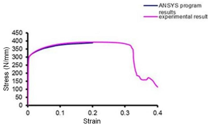
Fig. 12 Comparison between ANSYS program and experimental results of steel plate
