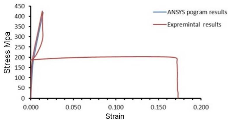
(c) Specimen with 4 layers of CFRP
