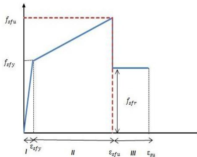
Fig. 14 Stress-strain relationship of SFCB
