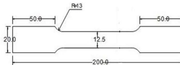
Fig. 2 Dimensions of test specimen
