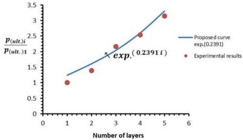
Fig. 15 Non-dimensional ultimate load of CFRP laminate versus CFRP layer numbers
