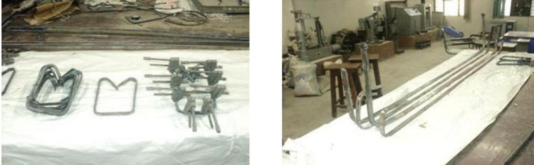
Fig. 1 Stirrups and longitudinal composite bars
