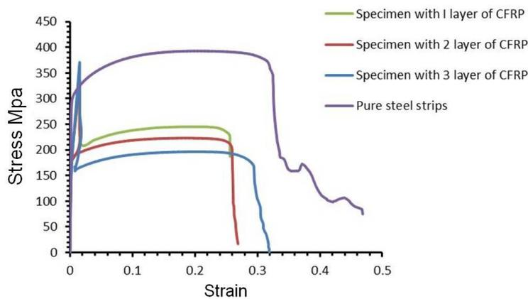
(a) Stress-strain curves of specimens with 1,2,3 layers of CFRP and pure steel strips
