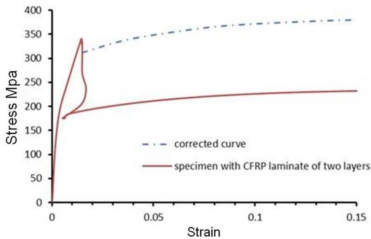
Fig. 16 Corrected stress-strain curve of specimen
