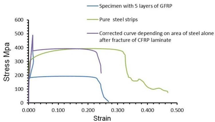
(b) Stress-strain curves of specimen with 5 layers of CFRP and pure steel strips
