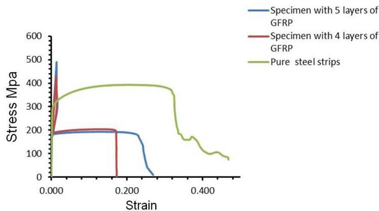
(b) Stress-strain curves of specimens with 4,5 layers of CFRP and pure steel strips
