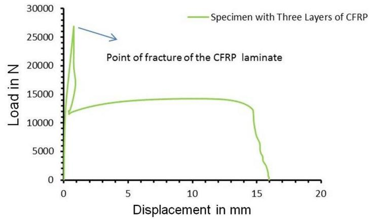
(d) Specimen with three layers of CFRP
