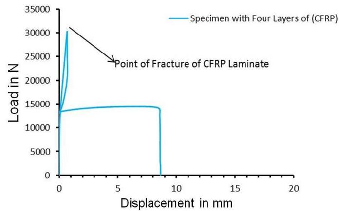
(e) Specimen with four layers of CFRP
