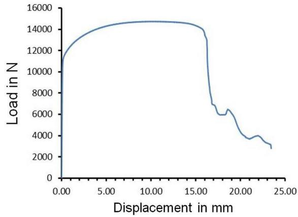
(a) Steel strips without CFRP
