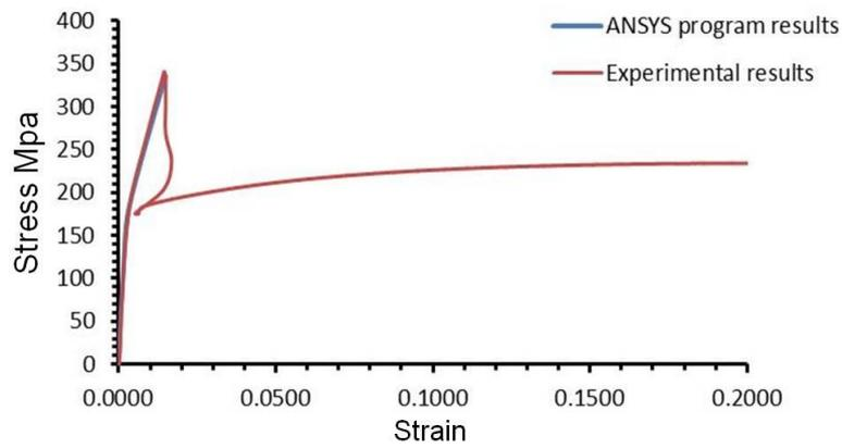
(a) Specimen with 2 layers of CFRP
