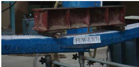
Fig. A3 Failure Pattern of beam FUW-L1(3)
