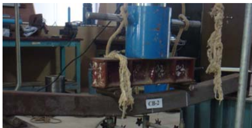
Fig. 5 Failure pattern of control beam
