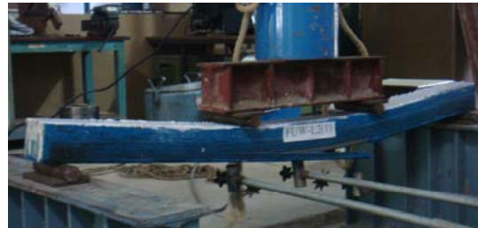
Fig. A4 Failure Pattern of beam FUW-L2(1)
