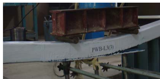
Fig. A8 Failure Pattern of beam PWB-L3(3)
