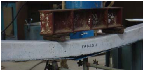
Fig. 9 Failure pattern of beam FWB-L2(1)
