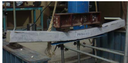
Fig. A6 Failure Pattern of beam PWB-L1(1)
