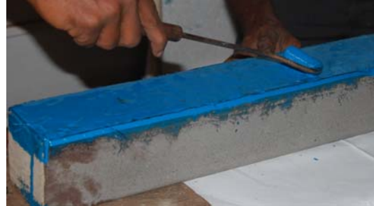
Fig. 2 Bonding of CFRP with the CFST specimen
