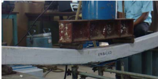
Fig. A1 Failure Pattern of beam FWB-L1(2)
