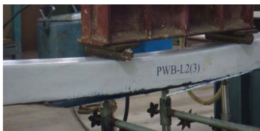
Fig. A7 Failure Pattern of beam PWB-L2(3)
