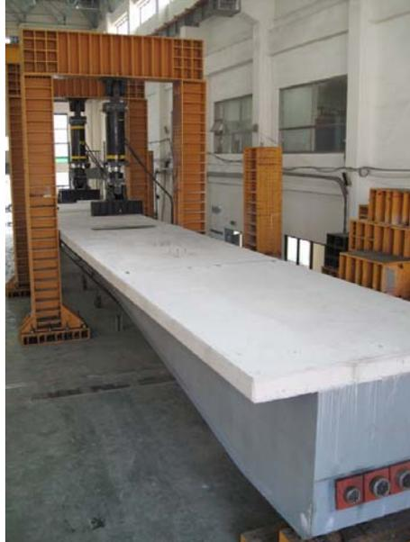
Fig. 9 Overview of static test setup
