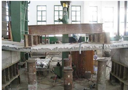
Fig. 4 Optical image of test setup for composite sandwich slabs
