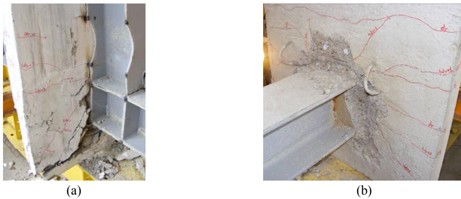
Fig. 30 (a) Failure of specimens DB-Comp1; and (b) DB-Comp 2
