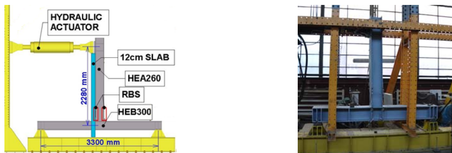
Fig. 19 Joint location and testing set-up
