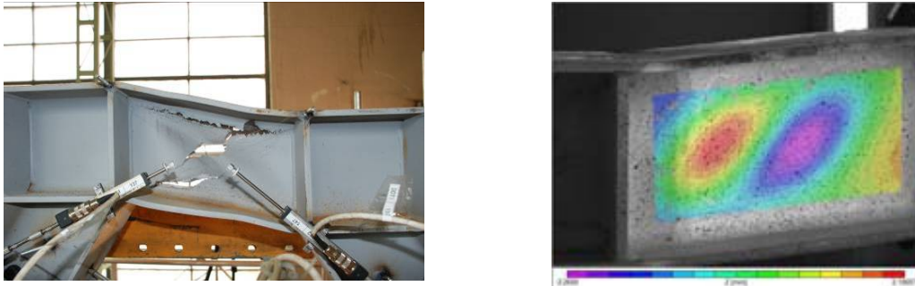
Fig. 12 Shear failure of EBF_M_LF-C link: pure deformation and strain deformation record for ultimate load
