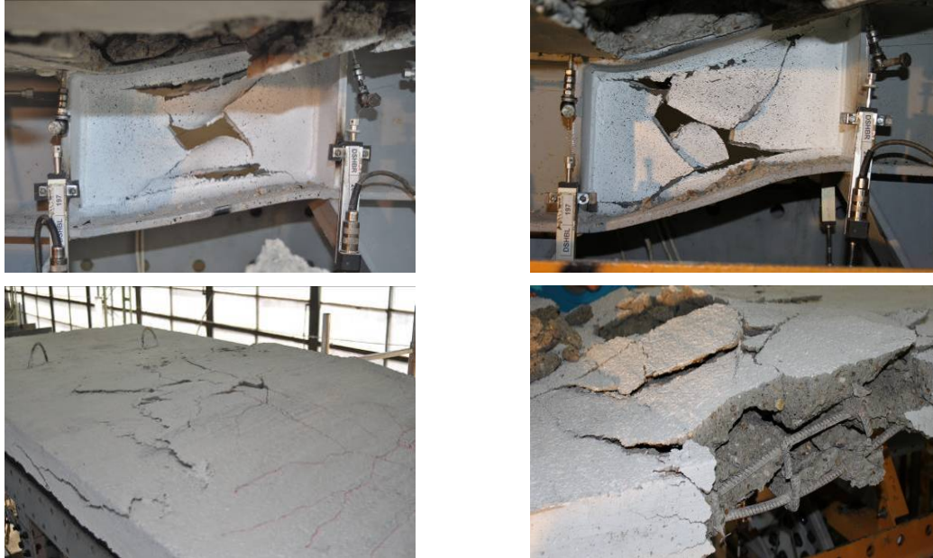
Fig. 16 Damage of the fixed link and concrete slab for EBF_LF_Comp1 (left) and Comp2 (right) specimens
