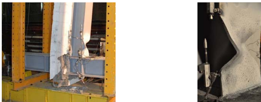
Fig. 34 Crushing of concrete and buckling of the compressed flange, and for the DB-Comp_RLD specimen
