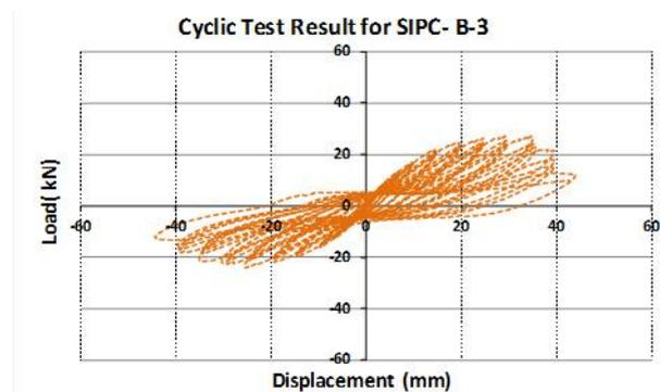
Fig. 11 Load-displacement for SIPC-B-3
