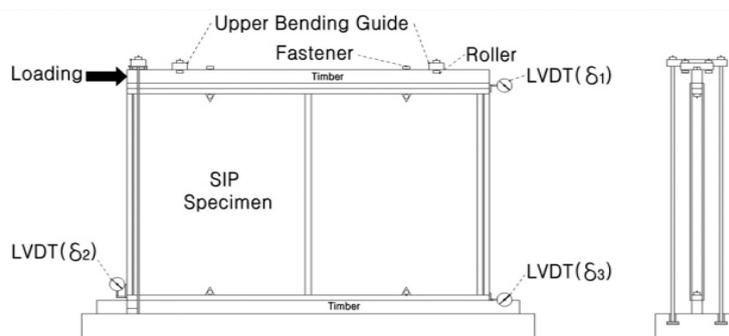
(b) Test setup for monotonic loading
