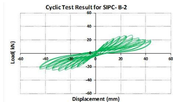
Fig. 10 Load-displacement for SIPC-B-2
