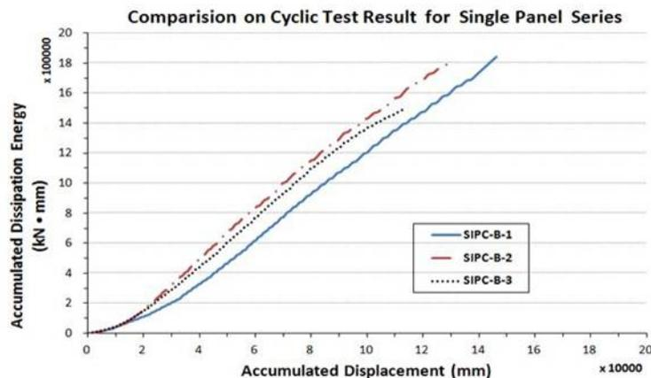
Fig. 19 Accumulated dissipation energy (SIPC-B)
