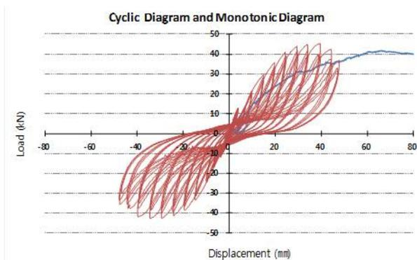
Fig. 18 Cyclic load-displacement with monotonic curve
