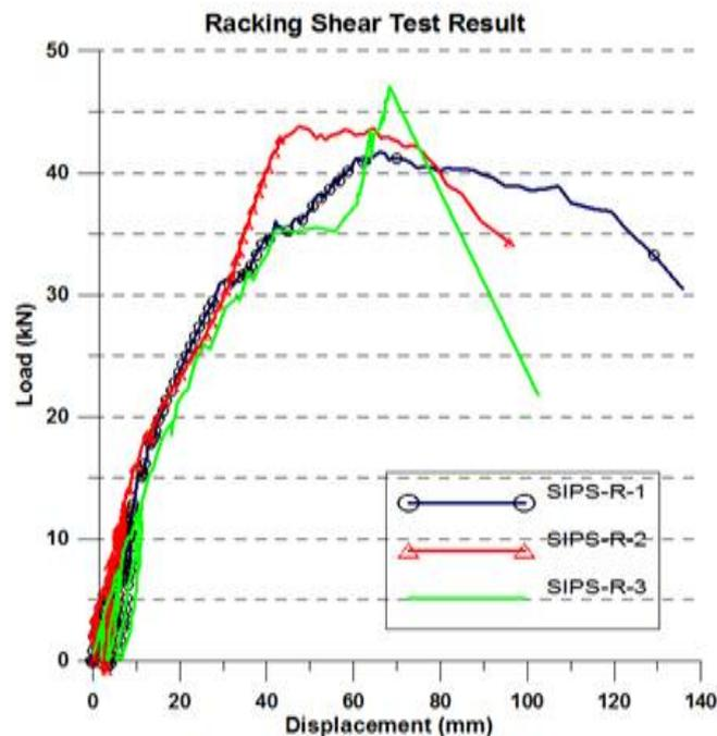
Fig. 4 Load-displacement of racking shear monotonic test result
