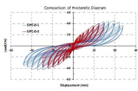
Fig. 8 Comparison between specimens for D-1 and D-3
