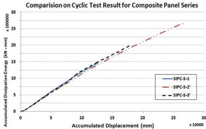
Fig. 20 Accumulated dissipation energy (SIPC-S)
