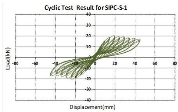
Fig. 13 Load-displacement for SIPC-S-1
