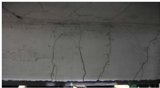
(a) Cracks of the pure bending segment
