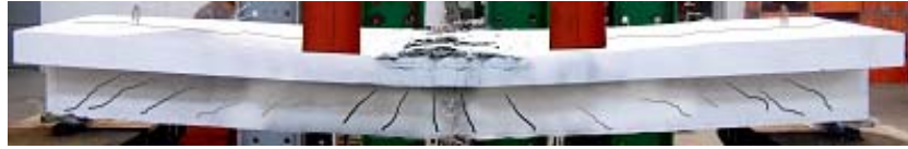
Fig. 6 Flexure failure (Shear span ratio = 3.1)
