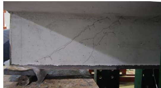
(b) Cracks of the flexure shear segment
