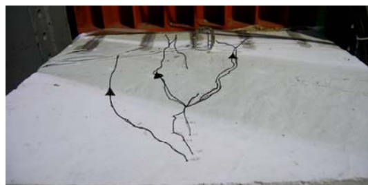
(c) Longitudinal cracks of deck
