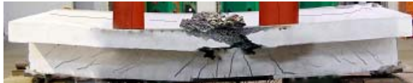
Fig. 7 Flexure failure (Shear span ratio = 2.0)
