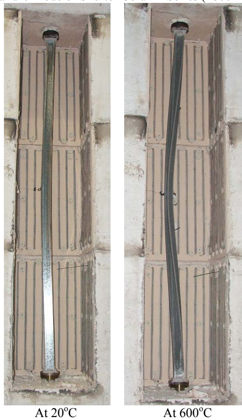
(b) Failure Mode of Longer Column Series (2800 mm)
