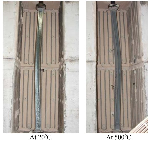
(a) Failure Mode of Shorter Column Series (1800 mm)
