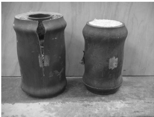
Fig. 7(a) Failure modes of unconfined CFST and CFST column
