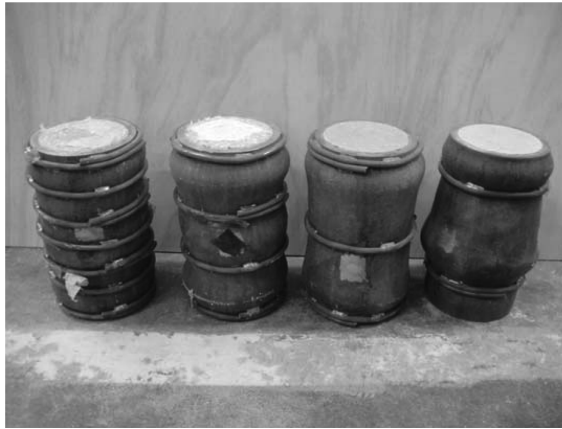
Fig. 7(c) Failure modes of CFST columns without external steel rings
