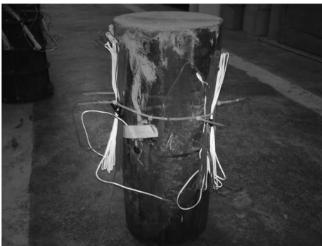
Fig. 1(c) CFST columns without external steel ring
