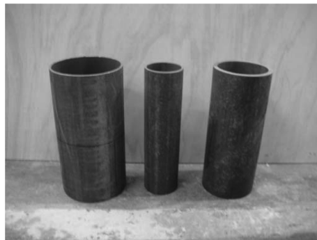
Fig. 1(e) Hollow steel tubes (Diameter = 168.3 mm, 88.9 mm and 139.7 mm)
