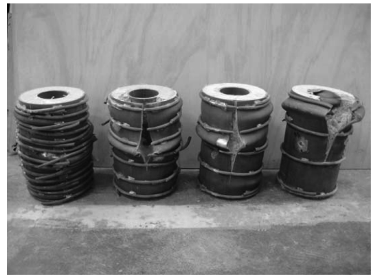
Fig. 7(b) Failure modes of CFDST columns with external steel rings
