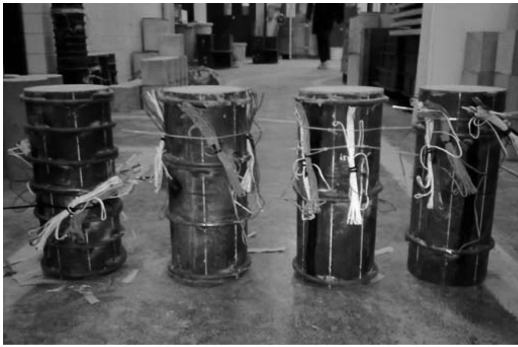
Fig. 1(a) CFST columns with external steel rings ( s=5t, 10t, 15t and 20t )
