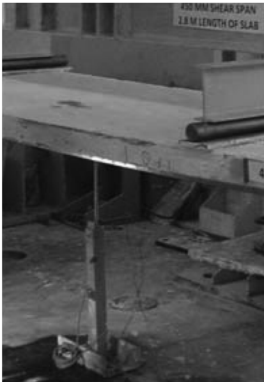
Fig. 5 LVDT at the mid span of the slab
