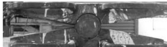
Fig. 7 Hinge Support used in experiment
