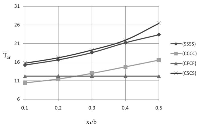
Fig. 3 Effect of the position of one intermediate line supports on the thermal buckling load for square laminated plates for different boundary conditions
