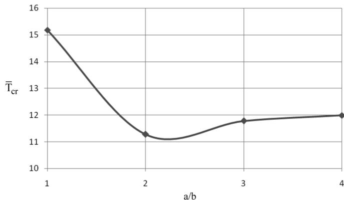
Fig. 9 Effect of plate aspect ratio on the critical thermal buckling load
