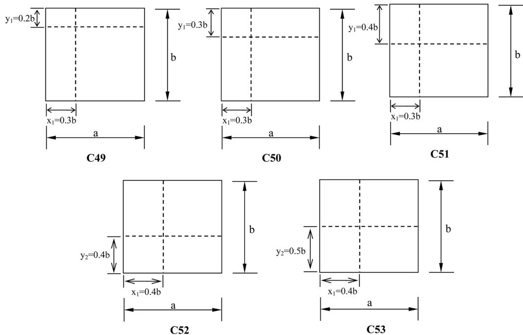
Fig. 2 53 different combinations of laminated plates with one or two intermediate line supports
