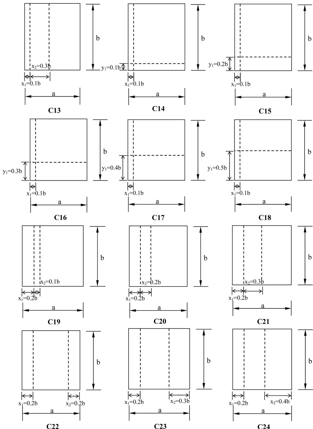
Fig. 2 53 different combinations of laminated plates with one or two intermediate line supports (Continued)
