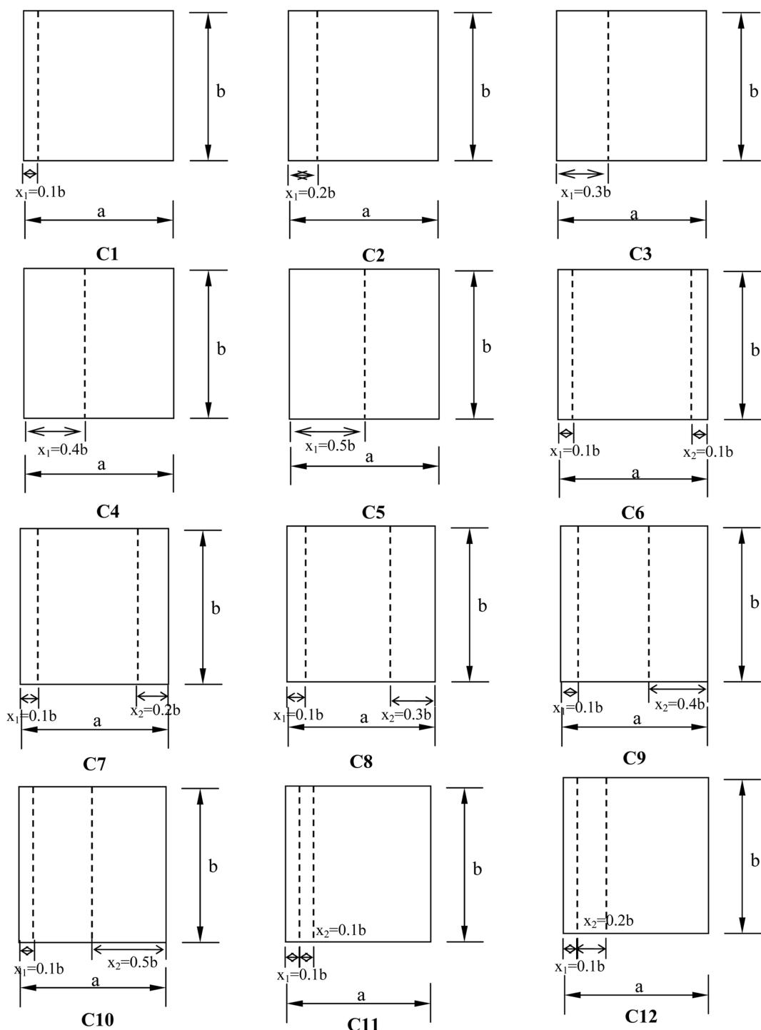
Fig. 2 53 different combinations of laminated plates with one or two intermediate line supports
