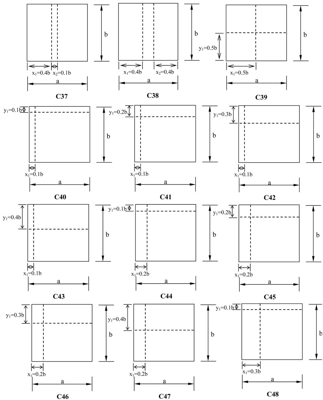
Fig. 2 53 different combinations of laminated plates with one or two intermediate line supports (Continued)
