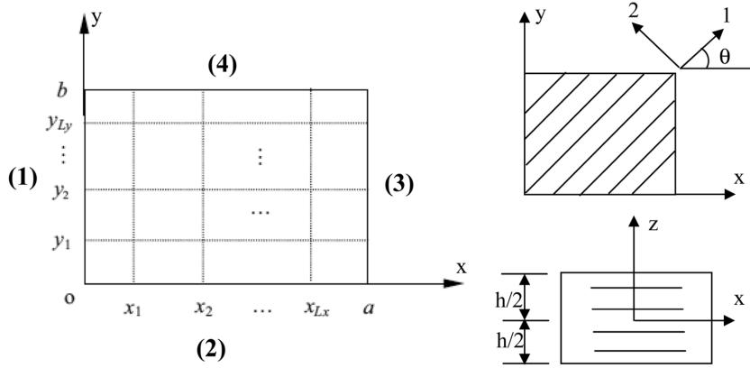
Fig. 1 Geometry of a rectangular laminated plate with internal line supports
