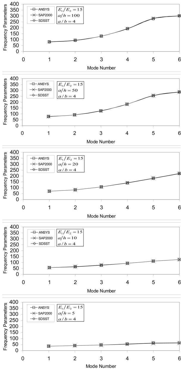
Fig. 7 Comparison of the frequency parameters of the first six modes obtained by SDSST and FEM (For Table 11-15)
