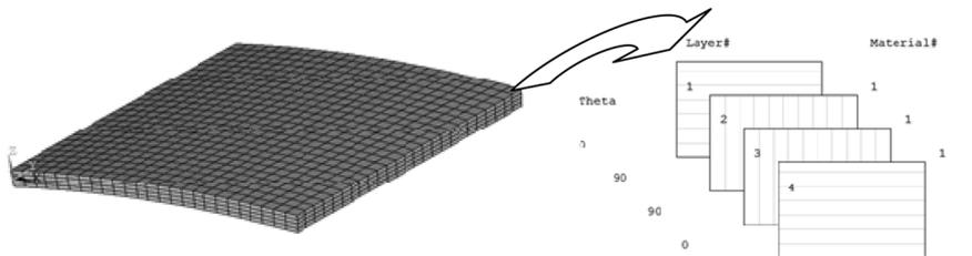
Fig. 3(b). Layered sequence for cylindrical shallow shell
