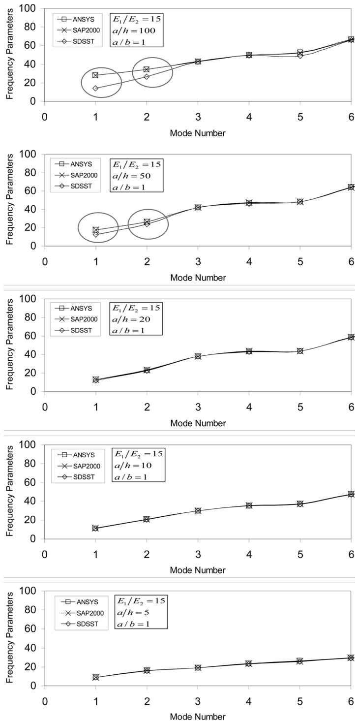
Fig. 5 Comparison of the frequency parameters of the first six modes obtained by SDSST and FEM (For Table 1-5)
