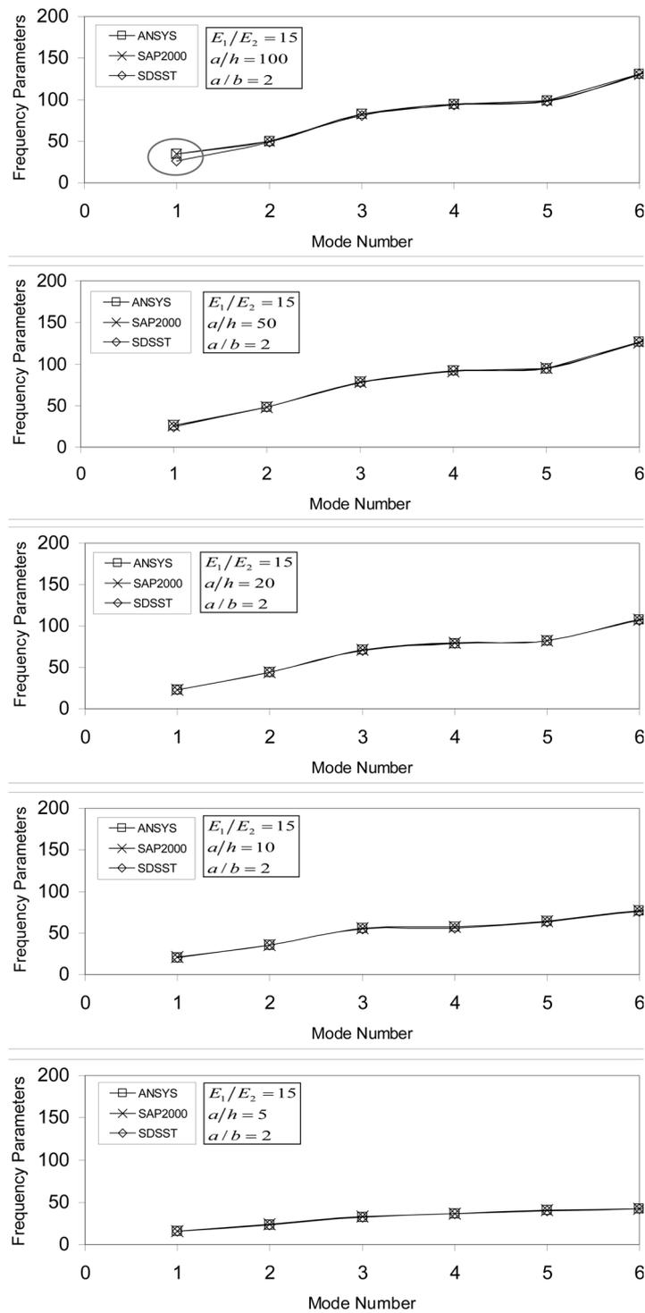
Fig. 6 Comparison of the frequency parameters of the first six modes obtained by SDSST and FEM (For Table 6-10)
