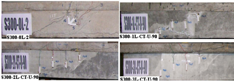
(b) Failure modes of tested beams-series-S300(U-Shape)
