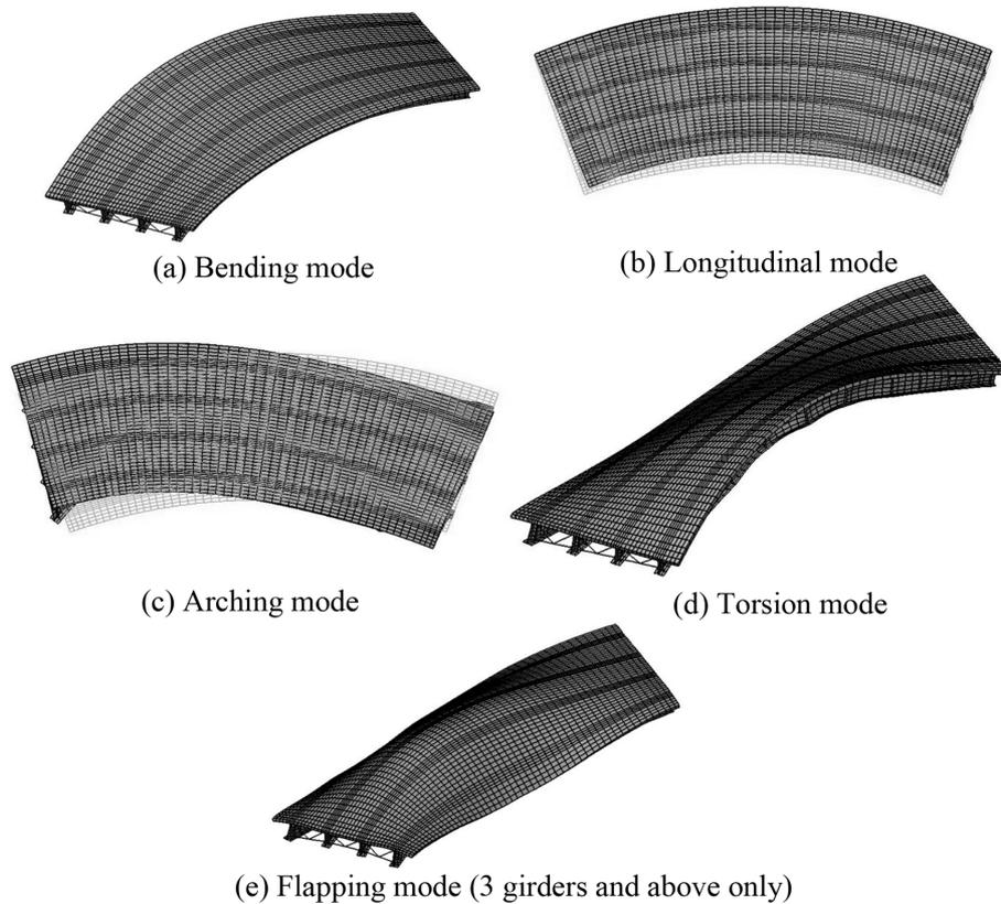
Fig. 11 Vibration mode shapes for curved composite bridge systems
