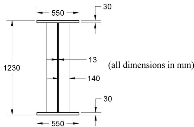
Fig. 4 Cross-section of the girders
