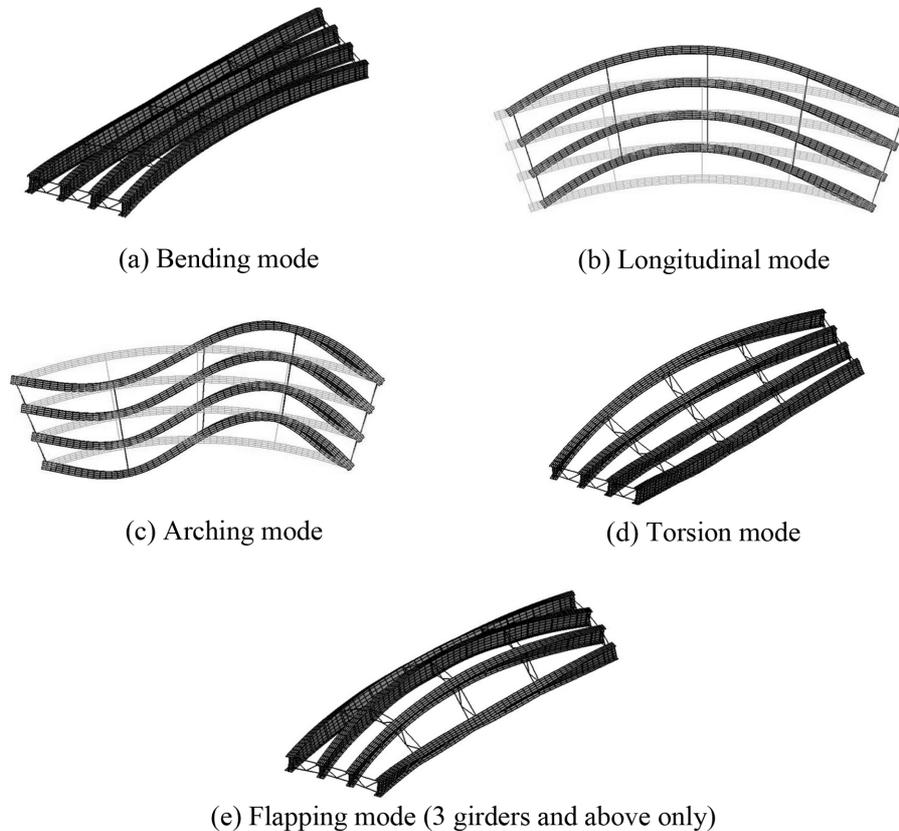
Fig. 9 Vibration mode Shapes for curved steel girder bridge systems
