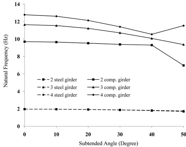
Fig. 14 Variation of natural frequency with subtended angle for longitudinal mode
