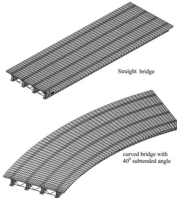
Fig. 1 Typical finite element mesh for composite girder bridges
