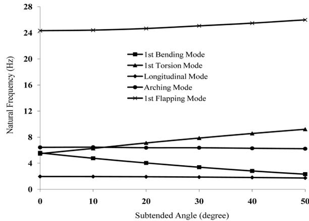
Fig. 17 Variation of natural frequency for 3- steel girder bridge system
