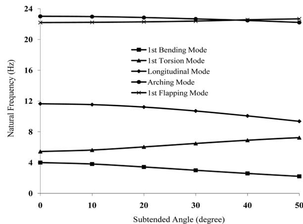
Fig. 18 Variation of natural frequency for 3- composite girder bridge systems
