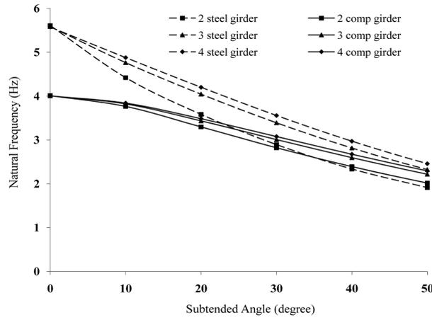
Fig. 12 Variation of natural frequency with subtended angle for first bending mode
