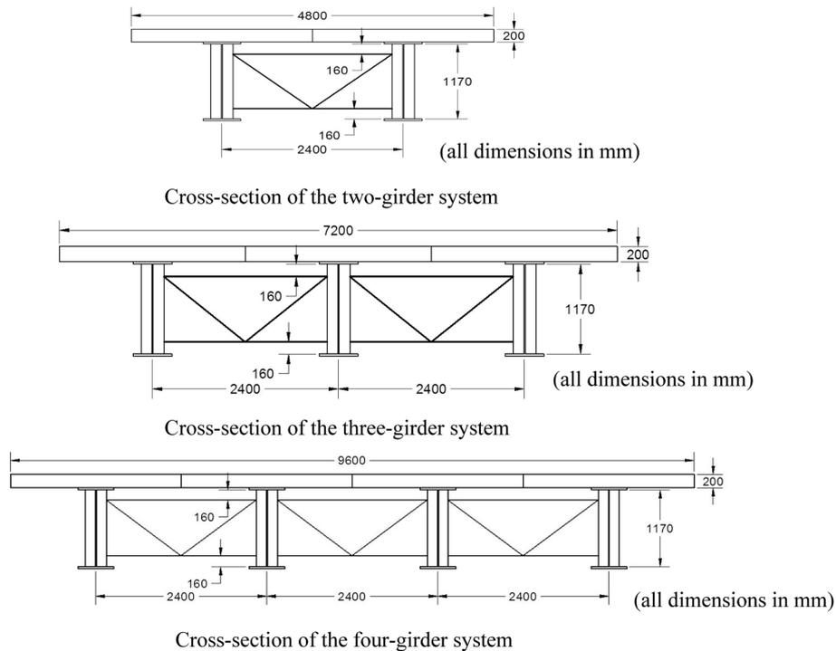
Fig. 5(a) Cross-section of different girder configurations
