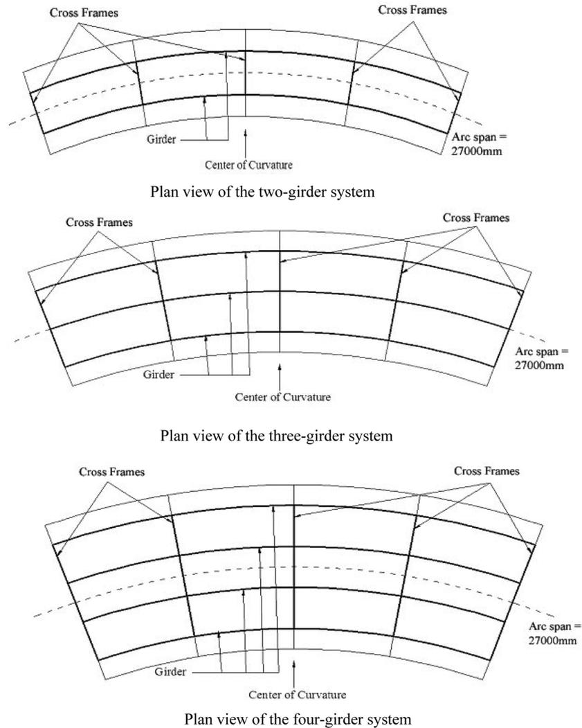
Fig. 5(b) Plan view of different girder configurations
