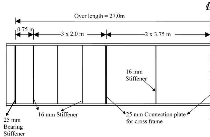
Fig. 6 Front elevation of a typical girder
