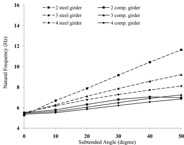
Fig. 13 Variation of natural frequency with subtended angle for first torsion mode
