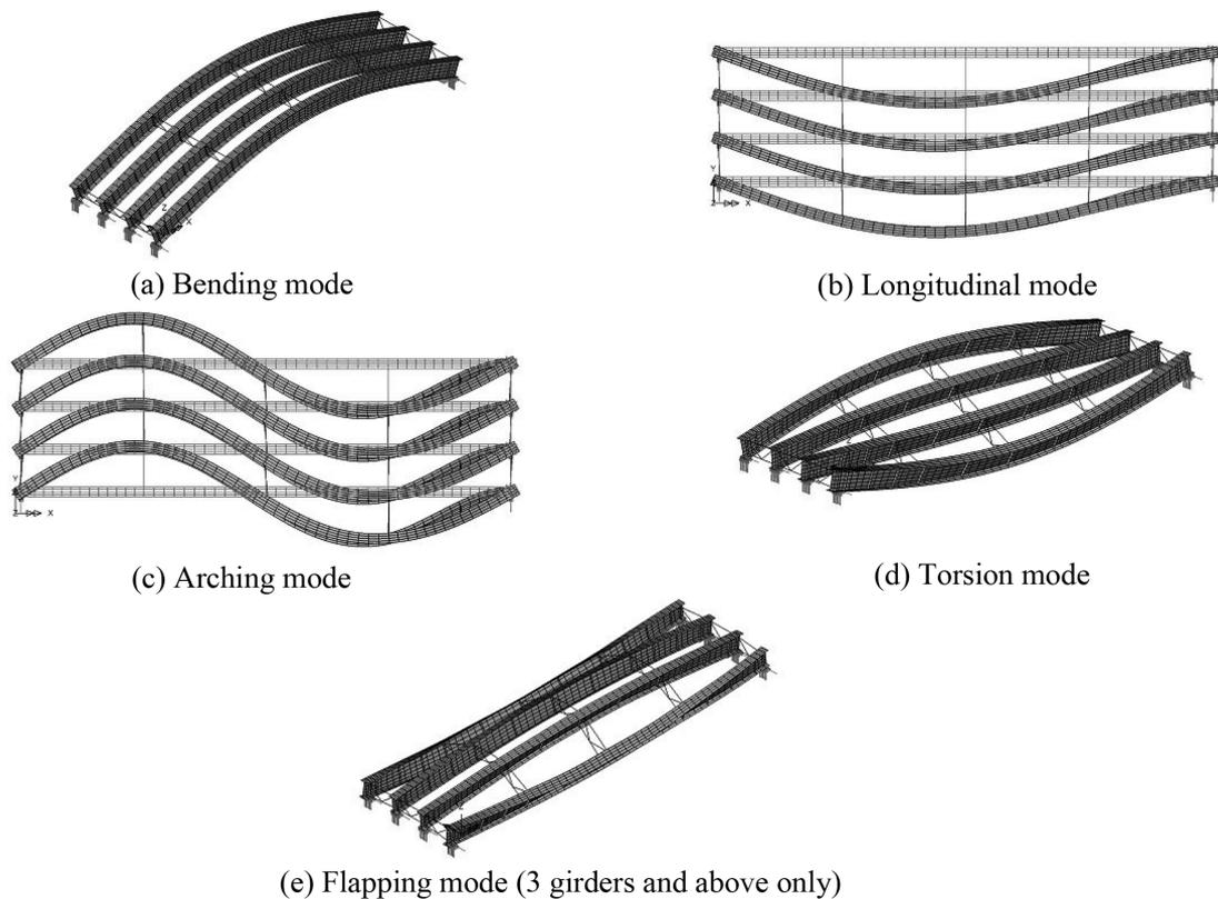
Fig. 8 Vibration mode Shapes for straight steel girder bridge systems
