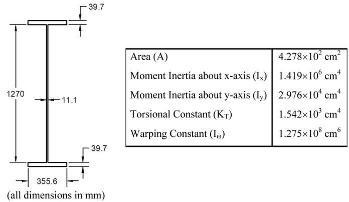
Fig. 2 Cross-section of the girder used by Yoon *et al.*(2005)
