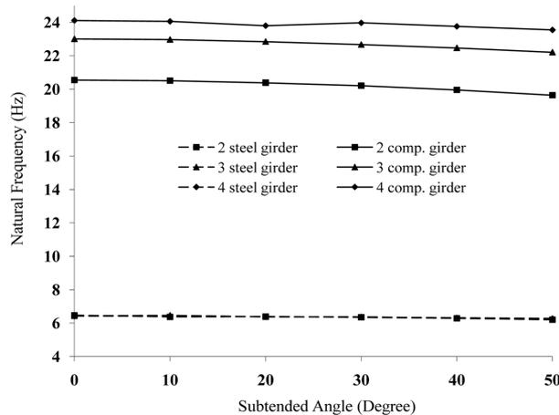
Fig. 15 Variation of natural frequency with subtended angle for arching mode
