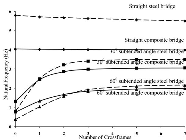
Fig. 7 Variation of natural frequency with number of intermediate cross-frames
