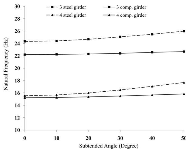
Fig. 16 Variation of natural frequency with subtended angle for flapping mode
