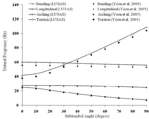
Fig. 3 Results for horizontally curved twin girders
