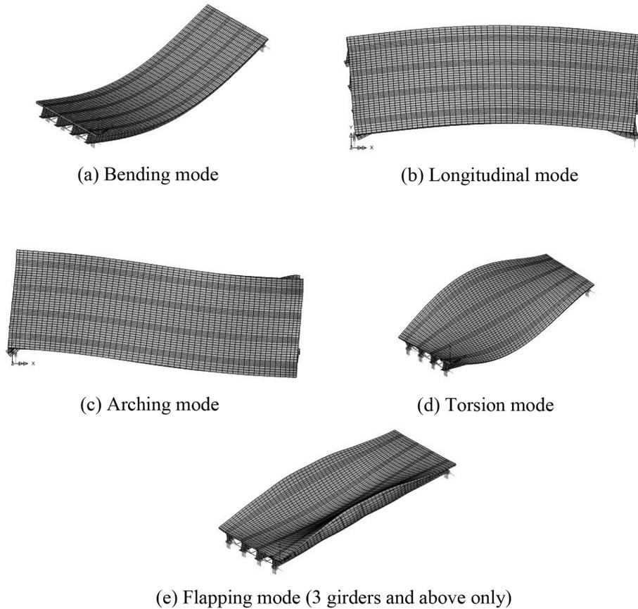
Fig. 10 Vibration mode shapes for straight composite bridge systems
