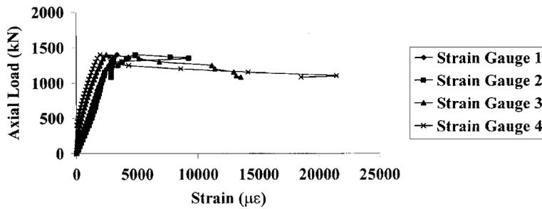
Fig. 11 Load-strain results of HSCI1
