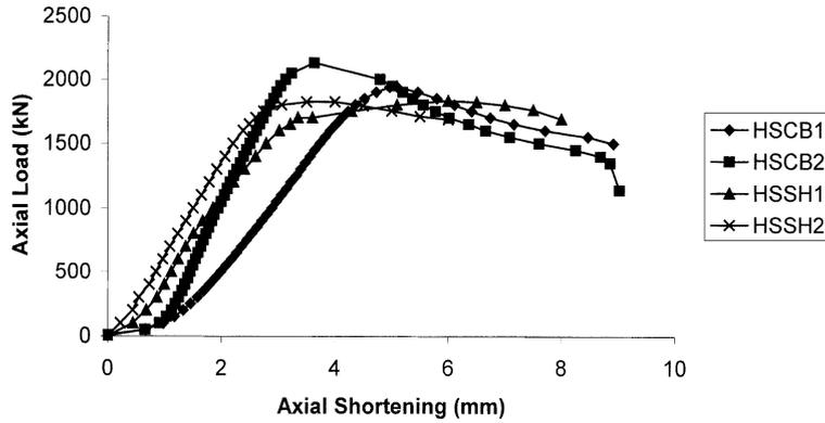
Fig. 10 Load-deflection results of fabricated box section columns
