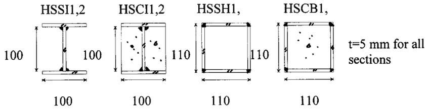
Fig. 3 Column cross-sections
