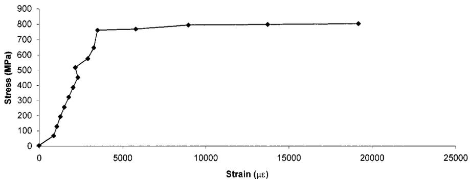
Fig. 6 Typical stress-strain curve for stub column
