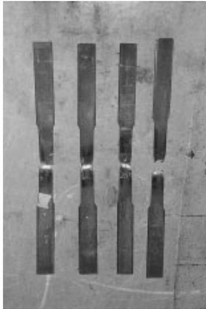
Fig. 5 Typical failure mode for tensile coupon
