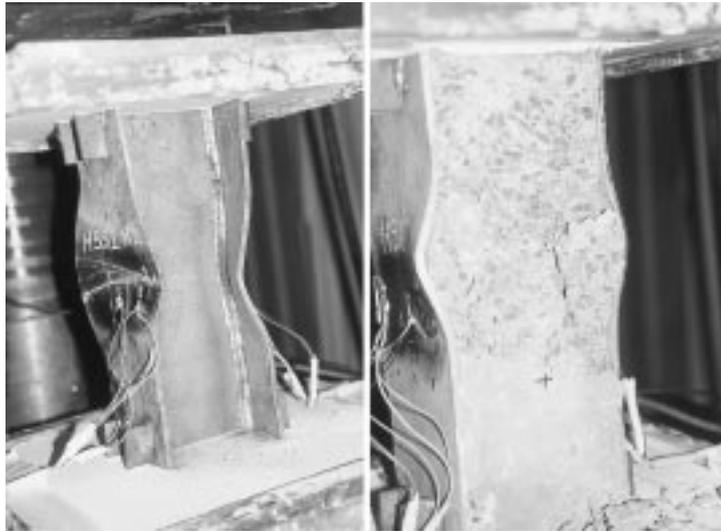
Fig. 13 Failure modes of columns
