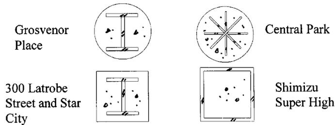
Fig. 2 High strength steel composite cross-sections
