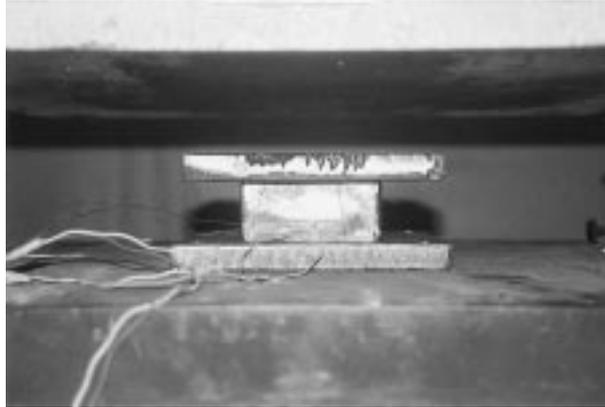
Fig. 7 Typical stub column failure
