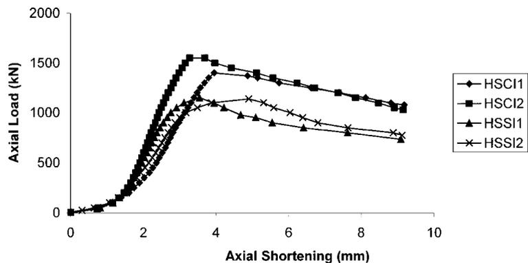
Fig. 9 Load-deflection results of fabricated I-section columns
