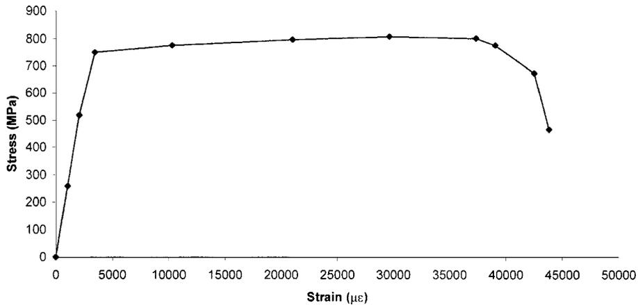
Fig. 4 Typical stress-strain curve for tensile coupon
