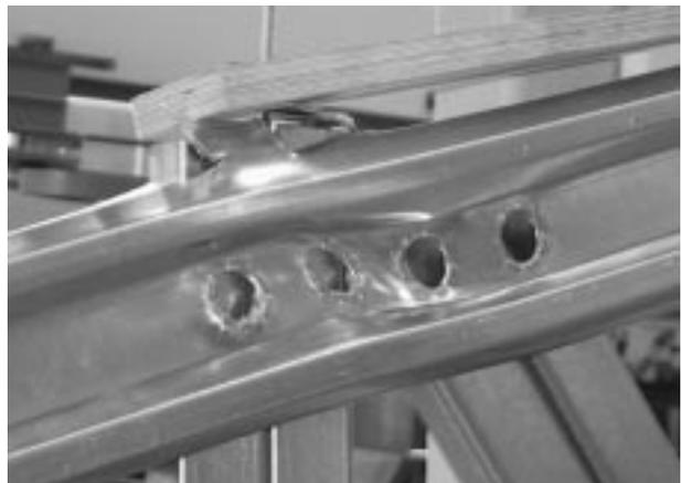
Fig. 18 Ruptured joints after test
