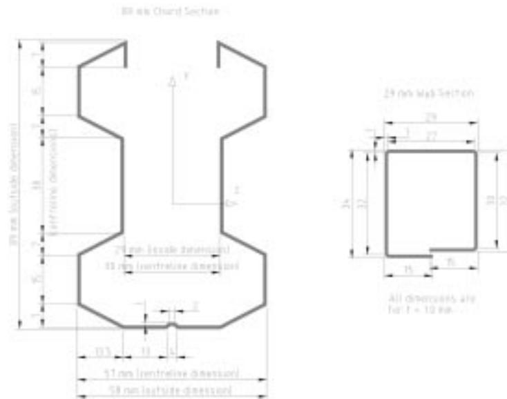
Fig. 5 The profiles used in the Rosette truss system
