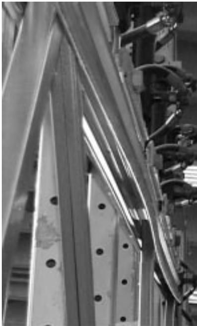
Fig. 17 Deformations of the top chord at total load value 39 kN
