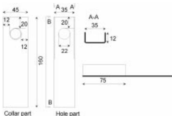
Fig. 6 Connected parts of test specimens in simple shear tests
