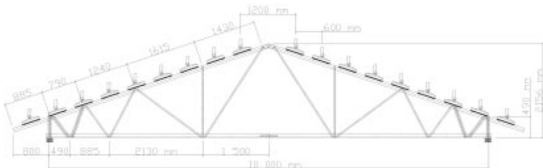
Fig. 11 Nominal geometry of test truss with load cylinders
