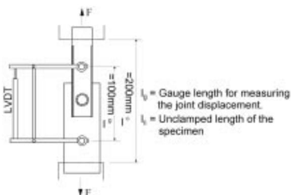
Fig. 7 Test set-up in simple shear test
