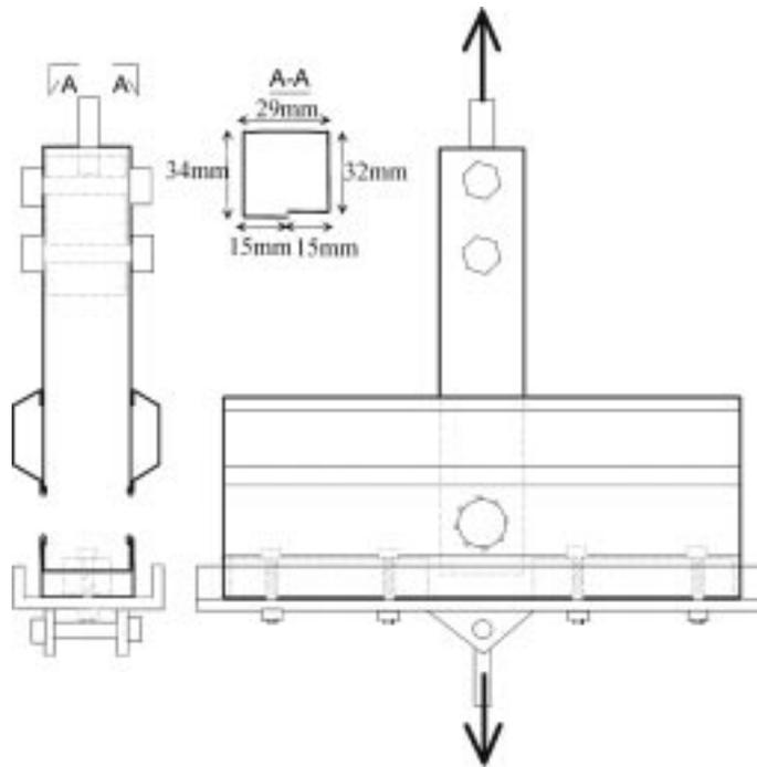
Fig. 9 T-connection test set-up in tension test
