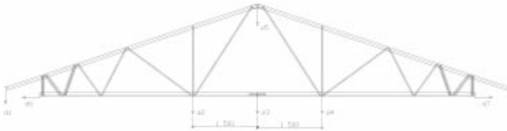
Fig. 15 Locations of displacement measurements
