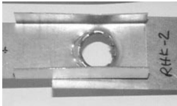
Fig. 8 Failure mode of simple shear test specimen
