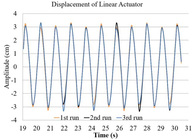
Fig. 2 Time series of linear actuator's displacement for three test runs (desired amplitude = 3 cm, filling ratio = 50%). Time range was recorded from 19 s to 31 s, which is coincident with  $T_i = 0$  s – 12 s, after fully ramping up
