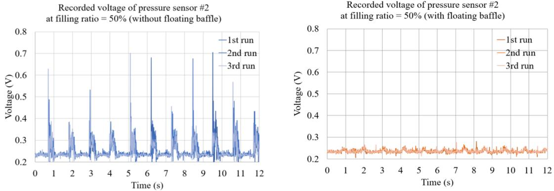
Fig. 12 Voltage recorded by pressure sensor at location S2 under sloshing by excitation with amplitude = 3.0 cm, period = 1.1 sec, and filling ratio 50%, (left) without floating baffle, and (right) with floating baffle
