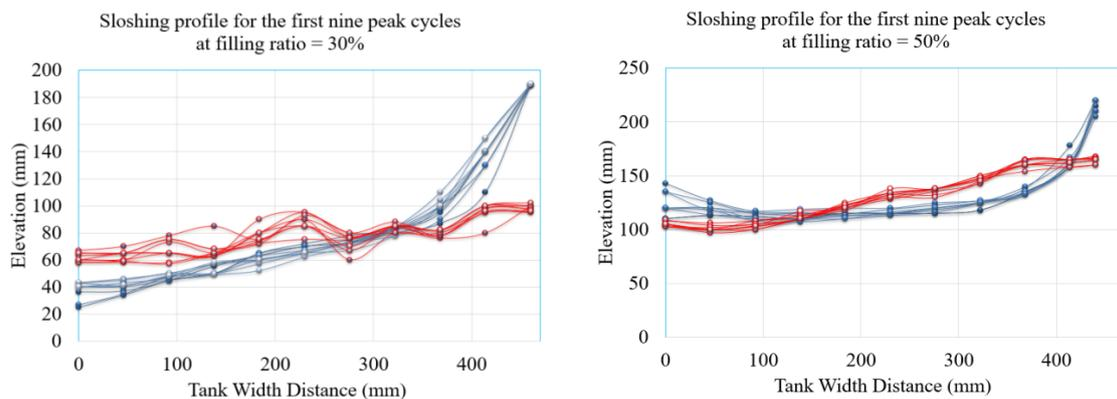
Fig. 9 Sloshing profile for first nine peaks of liquid under excitation with amplitude = 3.0 cm, period = 1.1 sec, (left) filling ratio = 30%, and (right) filling ratio = 50% (blue lines: without floating baffle, red lines: with floating baffle)
