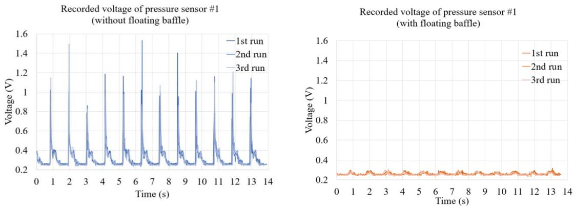
Fig. 10 Voltage recorded by pressure sensor at location s1 under sloshing by excitation with amplitude = 3.0 cm, period = 1.1 sec and filling ratio 30%, (left) without floating baffle, and (right) with floating baffle
