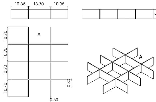
Fig. 4 Principal dimensions of model of floating baffle (unit in centimeter)
