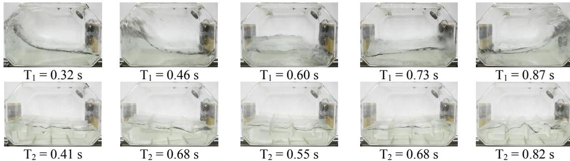
Fig. 5 First half-cycle of sloshing under excitation with amplitude = 3.0 cm, period = 1.1 sec, and filling ratio 30%, (upper) without floating baffle, and (bottom) with floating baffle
