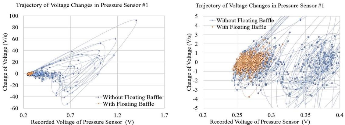
Fig. 11 Trajectory of voltage changes by pressure sensor at location S1 under sloshing by excitation with amplitude = 3.0 cm, period = 1.1 sec, and filling ratio 30%, (left) full view, and (right) zoom in view
