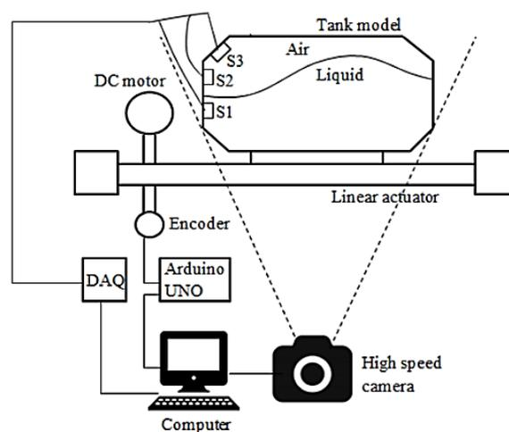
Fig. 1 Schematic drawing of sloshing experiment setup
