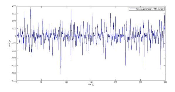
Fig. 14 Force acting on the MR damper at the 1<sup>st</sup> level
