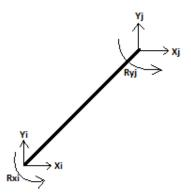
Fig. 4 Beam element in global coordinates
