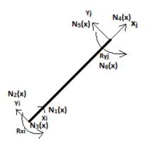
Fig. 3 Beam element in local coordinates
