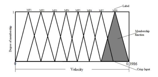
Fig. 8 Membership function for fuzzification of velocity
