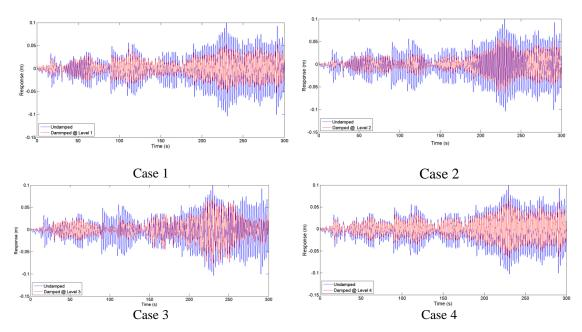
Fig. 15 MR damper placed at independent levels (cases - 1,2,3 &4)
