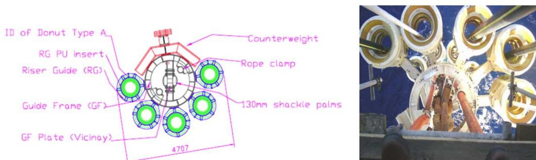
Fig. 2-1 Typical Schematic Diagram of Guide Frame
