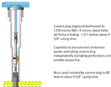
Fig. 3-5 Primary Cement Plug in Reservoir and Mechanical Barrier in Casing Section
