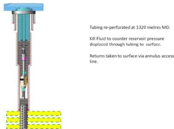
Fig. 3-7 Kill Fluid Displaced to Tubing & Annulus above Cement Plugs
