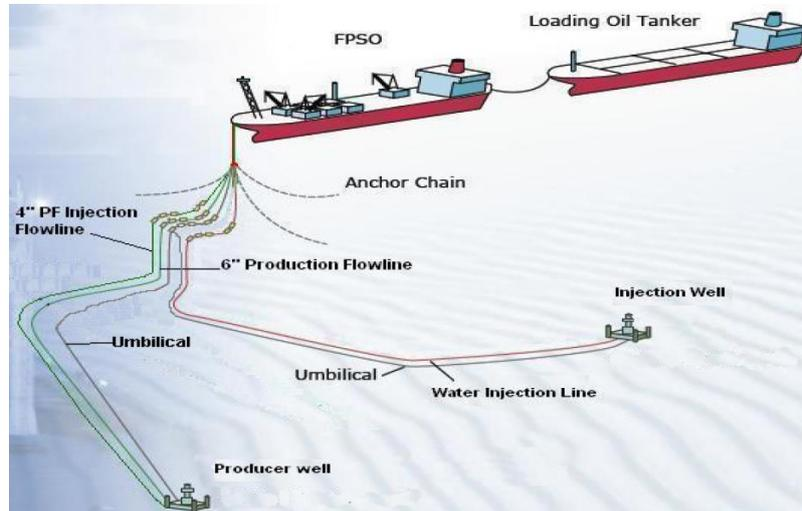
Fig. 1 The Layout of Oil Field Facilities and Subsea system
