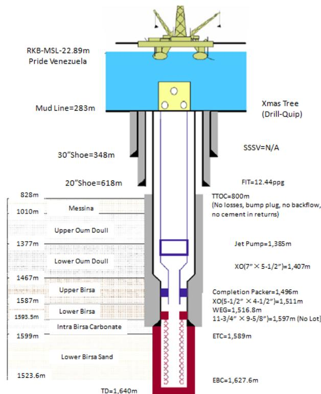
Fig. 3-2 Scheme of Producer Well (W-1)
