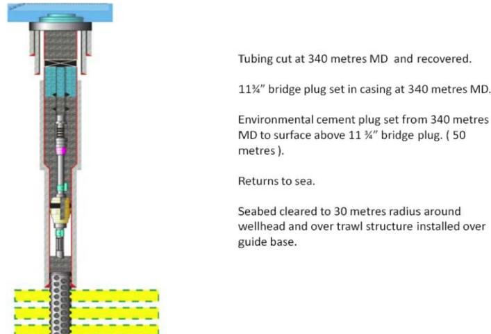
Fig. 3-8 Bridge Plug in Casing and Environmental Cement Plug Set
