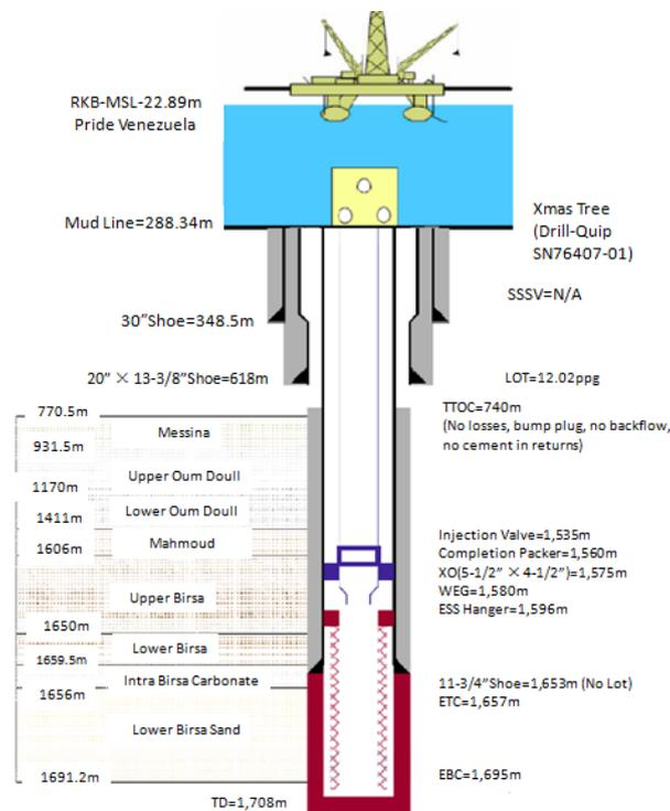
Fig. 3-3 Scheme of Injector Well (W-2)
