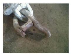
Fig. 1 The Anchor Chain Failure of Gryphon Alpha FPSO (Finucane 2012)
