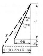
Fig. 2 The geometry of helical tendon before and after deformation
