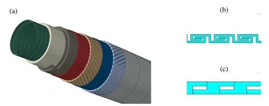
Fig. 2 Finite-element model of the flexible riser: (a) whole model, (b) carcass layer profile and (c) zeta layer profile
