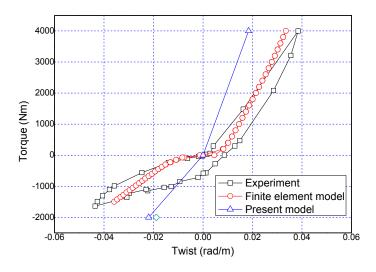
Fig. 4 Torque-twist relationship of the flexible riser with ends fixed axially
