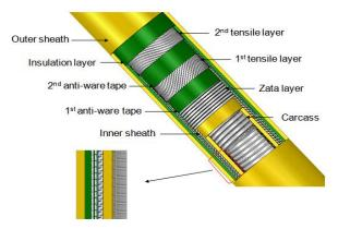
Fig. 1 Schematic diagram of a typical flexible riser
