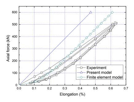
Fig. 3 Axial force-elongation relationship of the flexible riser with ends free to rotate
