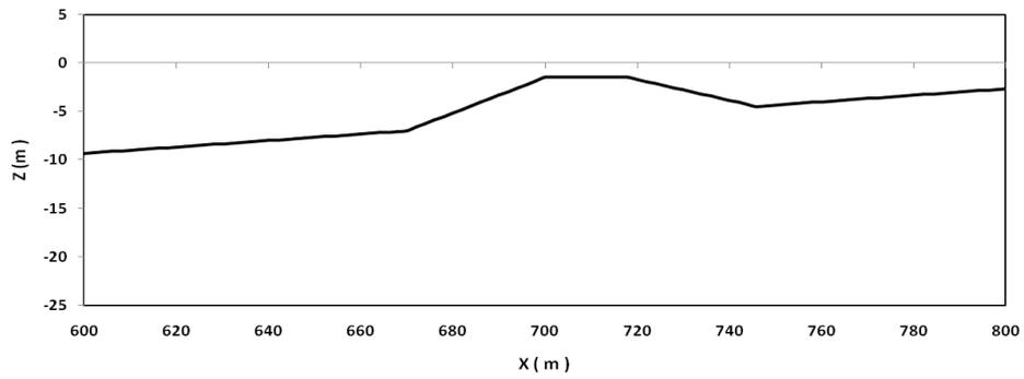
Fig. 3 A schematic of submerged breakwater surface
