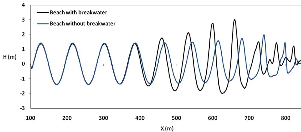
Fig. 9 Propagation of regular wave over beach at point  $Y=600$  m
