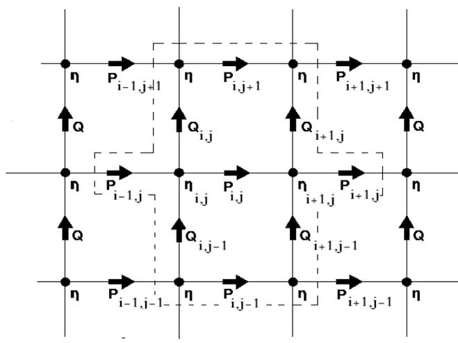
Fig. 1 Staggered grid notation in x-y space
