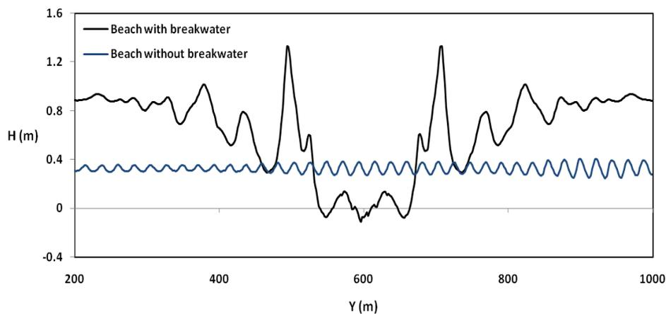
Fig. 10 Comparison of results of water level changes in the beach in lack of any structure and in presence of discontinuous submerged breakwater at point  $X=830$
