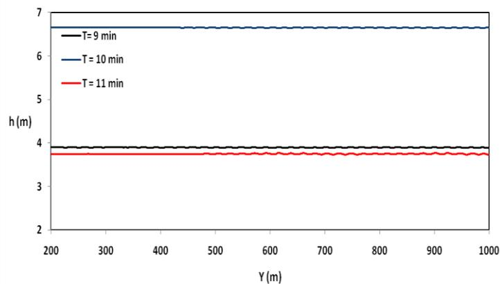
Fig. 6 Water depth elevation at point  $X = 740$  m on beach in the lack of breakwater
