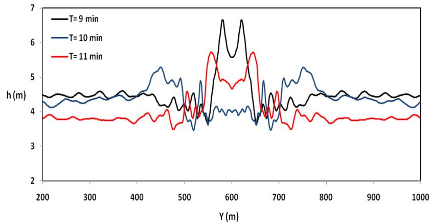
Fig. 7 Water depth elevation at point  $X=740$  m on beach in presence of discontinuous submerged breakwater
