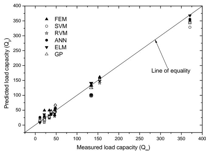
Fig. 2 Comparisons of predicted and measured uplift capacity of suction caisson by different models for testing data
