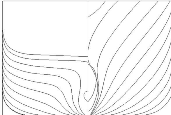
Fig. 7 Body Plan of C11 hull form
