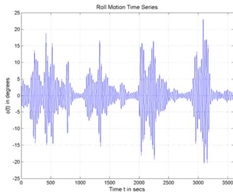
Fig. 12 Roll motion time series
