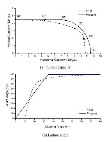
Fig. 2 Comparison with FEM simulations  $(H_p/D=6)$
