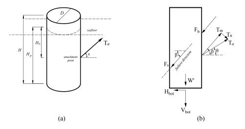
Fig. 1 Geometry and mechanical model of the suction anchor
