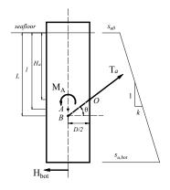
Fig. 6 Analytical method for predicting the optimal attachment point
