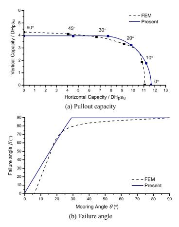
Fig. 3 Comparison with FEM simulations ( $H_p/D=10$ )
