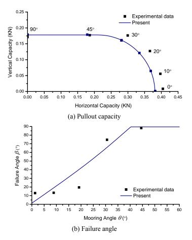
Fig. 5 Comparison with model tests
