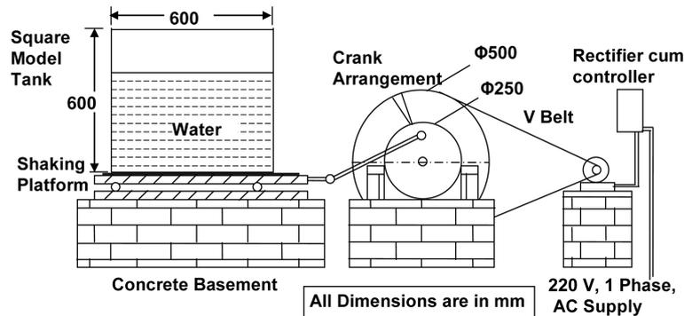
Fig. 1 A simple experimental setup for tank sloshing
