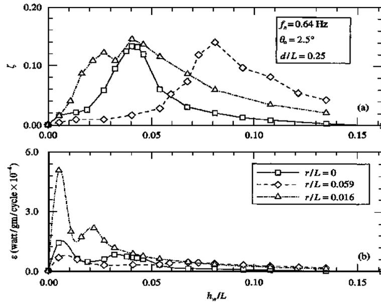
Fig. 9 Performance of the liquid damper as affected by the liquid height ( $h_w$ ) (Modi and Munshi 1998)
