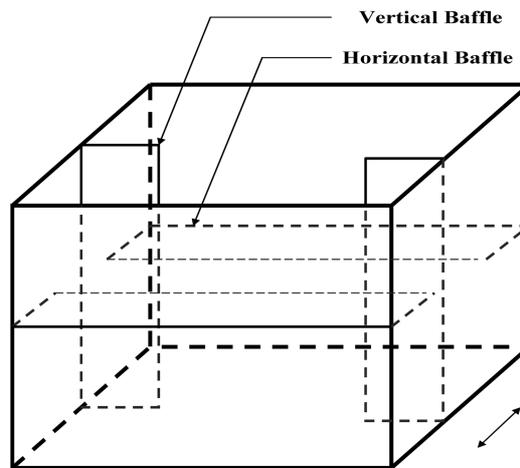
Fig. 5 Tank with vertical and horizontal baffles
