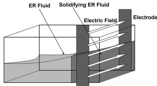
Fig. 11 Principle of ER-TSD (Sakamoto *et al.* 2001)
