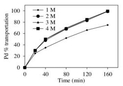
Fig. 8 Effect of HNO<sub>3</sub> concentration in feed solution on the transport of Pd(II); 1M-4M HNO<sub>3</sub> in feed solution, carrier: 0.01 M TETEDGA in n-dodecane, strippant: 0.02 M thiourea in 0.4 M HNO<sub>3</sub>, membrane: 0.2  $\mu$ m PTFE
