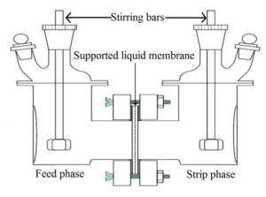
Fig. 2 Schematic diagram for flat sheet supported liquid membrane (FSSLM)
