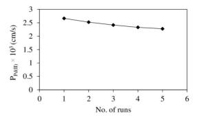
Fig. 11 Stability of SLM, number of runs versus permeability coefficient;  $[HNO_3] = 3$  M in feed solution, carrier: 0.01 M TETEDGA in n-dodecane, strippant: 0.02 M thiourea in 0.4 M HNO<sub>3</sub>, membrane: 0.2  $\mu$ m PTFE
