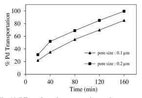
Fig. 10 Effect of membrane pore size on the transport of Pd(II);  $[HNO_3] = 3 M$  in feed solution, carrier: 0.01 M
