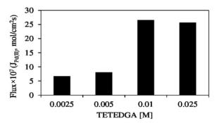
Fig. 9 Effect of TETEDGA concentration on the initial flux value of Pd(II); [HNO<sub>3</sub>] = 3M, strippant: 0.02M thiourea in 0.4 M HNO<sub>3</sub>, membrane: 0.2  $\mu$ m PTFE
