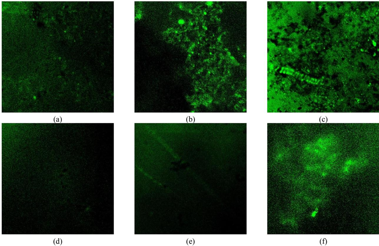
Fig. 3 The CLSM images of biofilm from the reactors w/o (above) or with (below) NAC addition at different MLSS concentrations: (a) and (d) 2500 mg/L, (b) and (e) 5200 mg/L, and (c) and (f) 8200 mg/L
