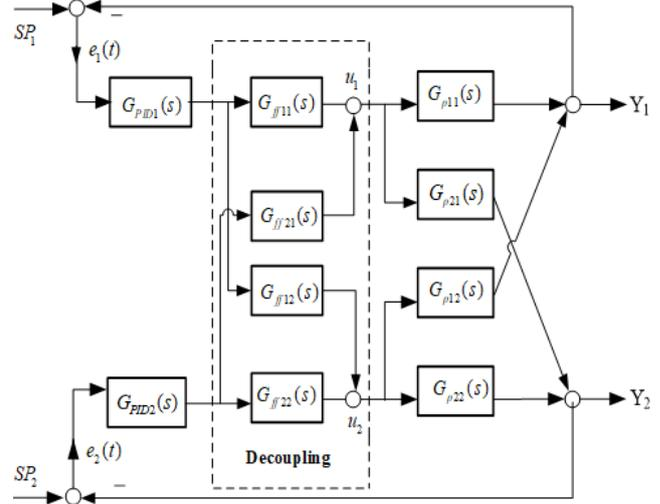
Fig. 2 Decoupling control system for RO system
