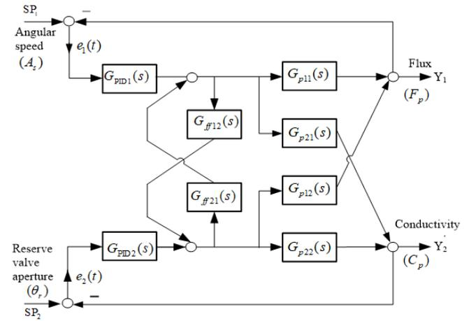
Fig. 3 Total decoupled scheme of an RO system with 2-PID controllers
