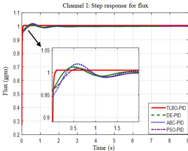
Fig. 6 Step response of flux (gpm) for channel I
