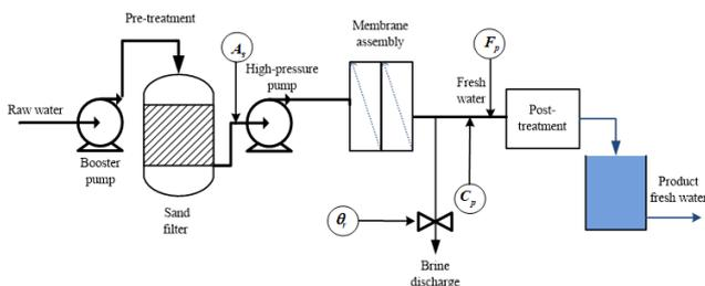
Fig. 1 A schematic block diagram of RO system water is stabilized with adjustment in pH level in the range
