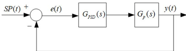
Fig. 4 A common feedback control system with PID controller
