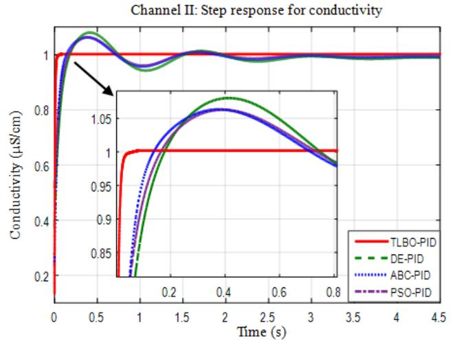
Fig. 7 Step response of conductivity(µS/cm) for channel II
