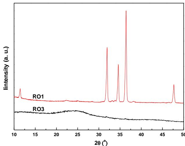
Fig. 7 X-ray diffractograms of different NF membranes
