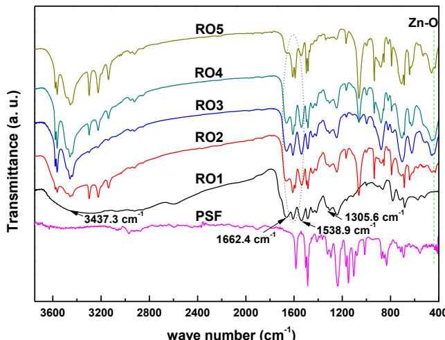
Fig. 4 FTIR spectra of different membranes
