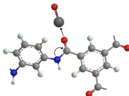
Fig. 5 Illustration of the interaction between C=O groups in polyamide chains and ZnO nanospheres
