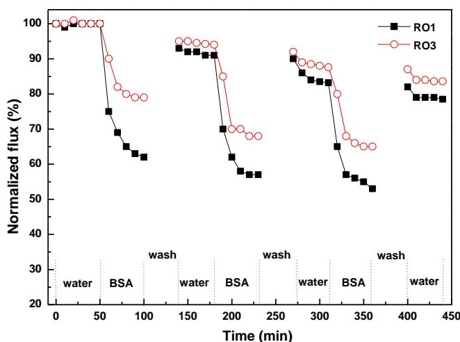
Fig. 12 Time-dependent normalized flux of the virgin and modified RO membranes
