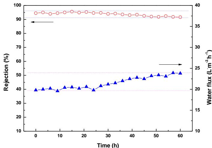
Fig. 11 The stability of separation performance of TFN RO membrane (RO3) ( $1 \text{ g}\cdot\text{L}^{-1}$  NaCl aqueous solution at  $0.7 \text{ MPa}$ ,  $25^\circ\text{C}$  for  $60 \text{ h}$ )
