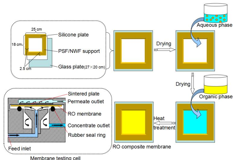
Fig. 2 The preparation flow scheme of RO composite membrane and the configuration of membrane testing cell
