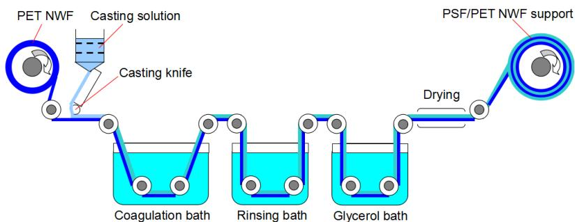
Fig. 1 The schematic diagram of the preparation of PSF/PET NWF support
