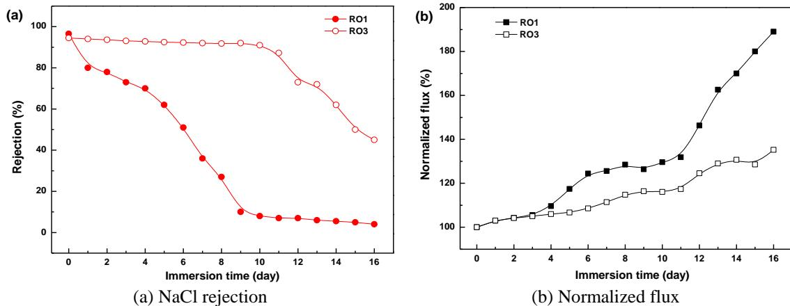
Fig. 13 Variations of different RO membrane separation performance after the exposure to 100 ppm NaClO (pH=6.5)
