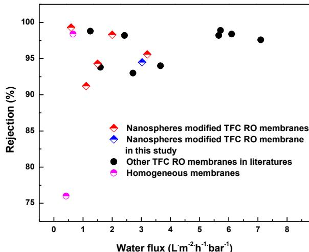
Fig. 10 Relationship between water flux and NaCl rejection of various RO membranes
