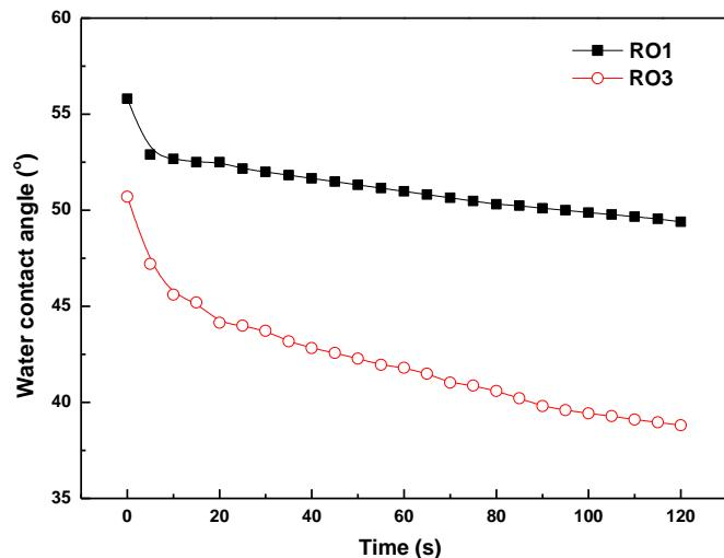
Fig. 8 Dynamic water contact angle of different NF membrane
