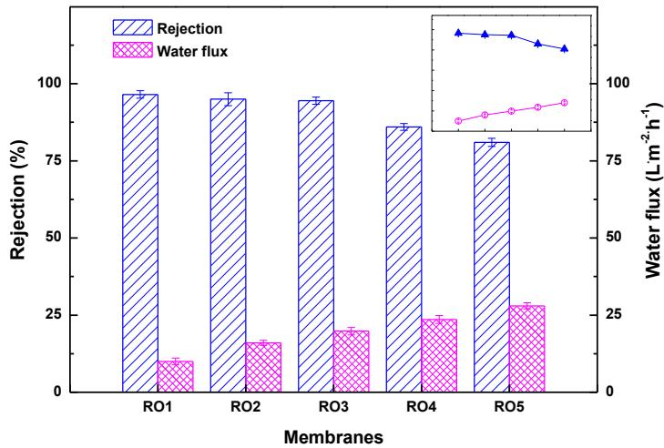
Fig. 9 Salt rejection and water flux of the virgin and modified RO membranes tested with  $1 \text{ g L}^{-1}$  NaCl aqueous solution at  $25^\circ\text{C}$  and  $0.7 \text{ MPa}$
