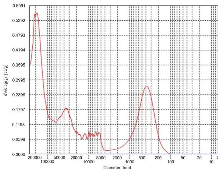
Fig. 3 Pore size distribution of PSF/NWF support membrane
