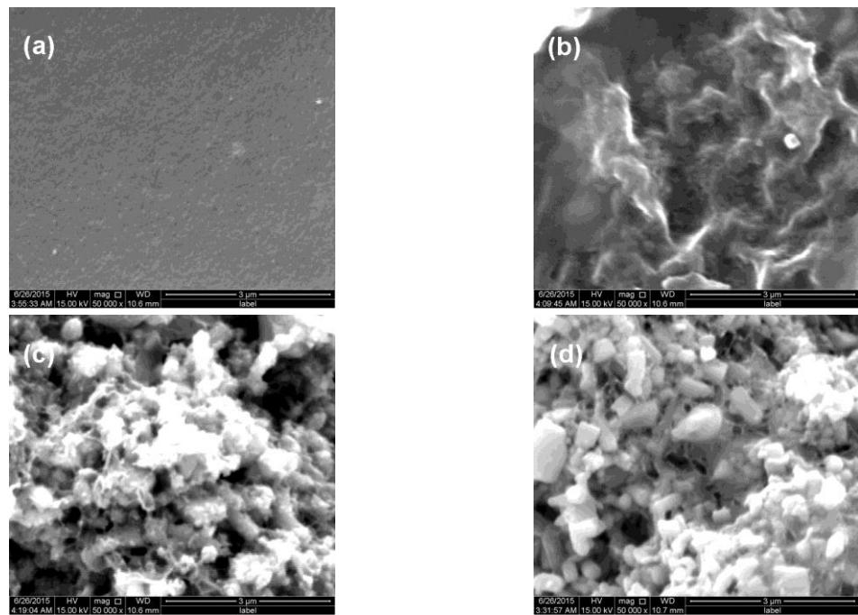
Fig. 6 SEM images of different membrane surface (a) PSF support membrane; (b) RO1; (c) RO3; (d) RO5
