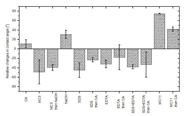
Fig. 2 Changes in contact angle values of the ESPA2 membrane as a consequence of single and sequential chemical cleaning. A positive value indicates an increase in the hydrophobicity, and vice versa. The measurements were conducted at room temperature (ca. 25°C) with Milli-Q water used as a reference solvent. The error bars show the standard deviation of five replicated measurements
