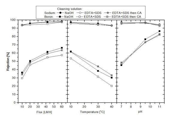
Fig. 8 Changes in boron and sodium rejections by the ESPA2 membrane after membrane cleaning with EDTA + SDS solution (pH 11) and EDTA + SDS solution followed by citric acid solution (pH 3). Unless otherwise stated, the testing conditions are: pH 8, feedwater contains 0.43 mM B(OH)<sub>3</sub>, 10 mM NaCl, 1 mM NaHCO<sub>3</sub>, and 1 mM CaCl<sub>2</sub>; temperature 20°C, permeate flux 20 LMH, cross-flow velocity 42 cm.s<sup>-1</sup>
