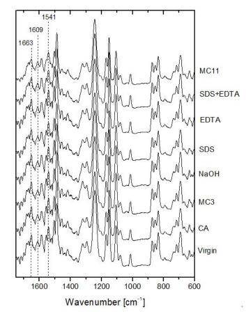
Fig. 3 FTIR absorption spectra of virgin and chemically cleaned ESPA2 membranes at 2 cm<sup>-1</sup> resolution
