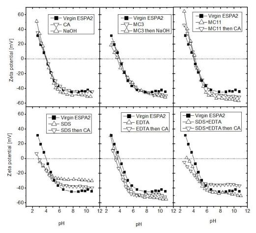
Fig. 1 Changes in zeta potential of the ESPA2 membrane as a consequence of single and sequential chemical cleaning. The measurements were conducted at room temperature (ca. 25°C) in a 1 mM KCl solution
