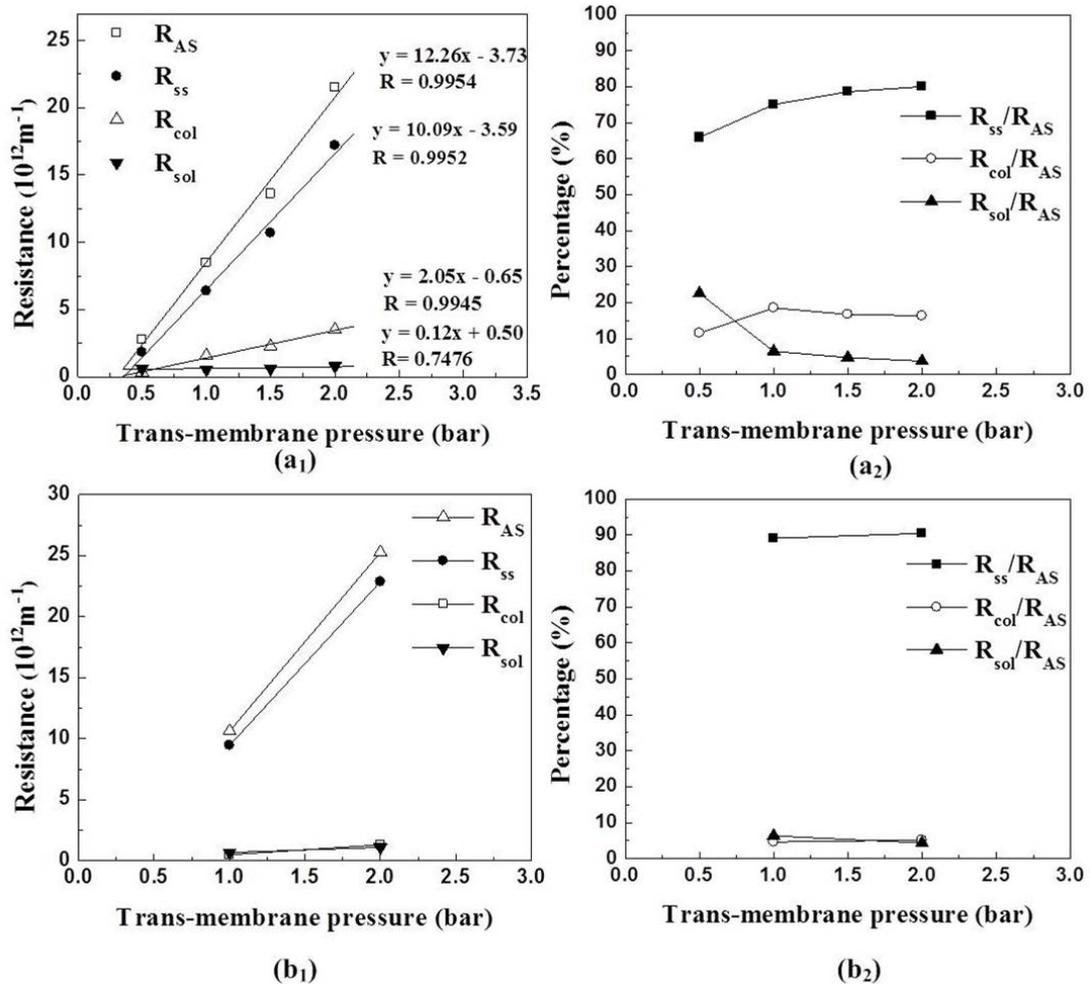
Fig. 4 Resistances of different sludge fractions according to trans-membrane pressure (a<sub>1</sub>), (a<sub>2</sub>) MBR; (b<sub>1</sub>), (b<sub>2</sub>) SBR (MLSS = 320 mg/L, CFV = 0.156 m/s)
