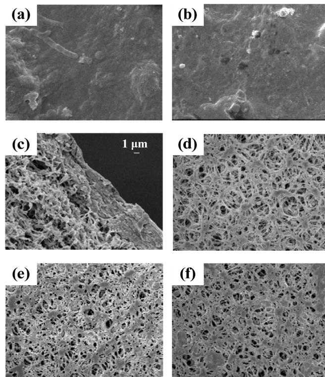
Fig. 6 Images of membrane morphology: (a) Fouled membrane (MBR, 8000 $\times$ ); (b) Fouled membrane (SBR, 8000 $\times$ ); (c) Fouled membrane (MBR, cross section, 4500 $\times$ ); (d) New membrane (4000 $\times$ ); (e) Fouled membrane after physical cleaning (MBR, 4000 $\times$ ); (f) Fouled membrane after physical cleaning (SBR, 4000 $\times$ )
