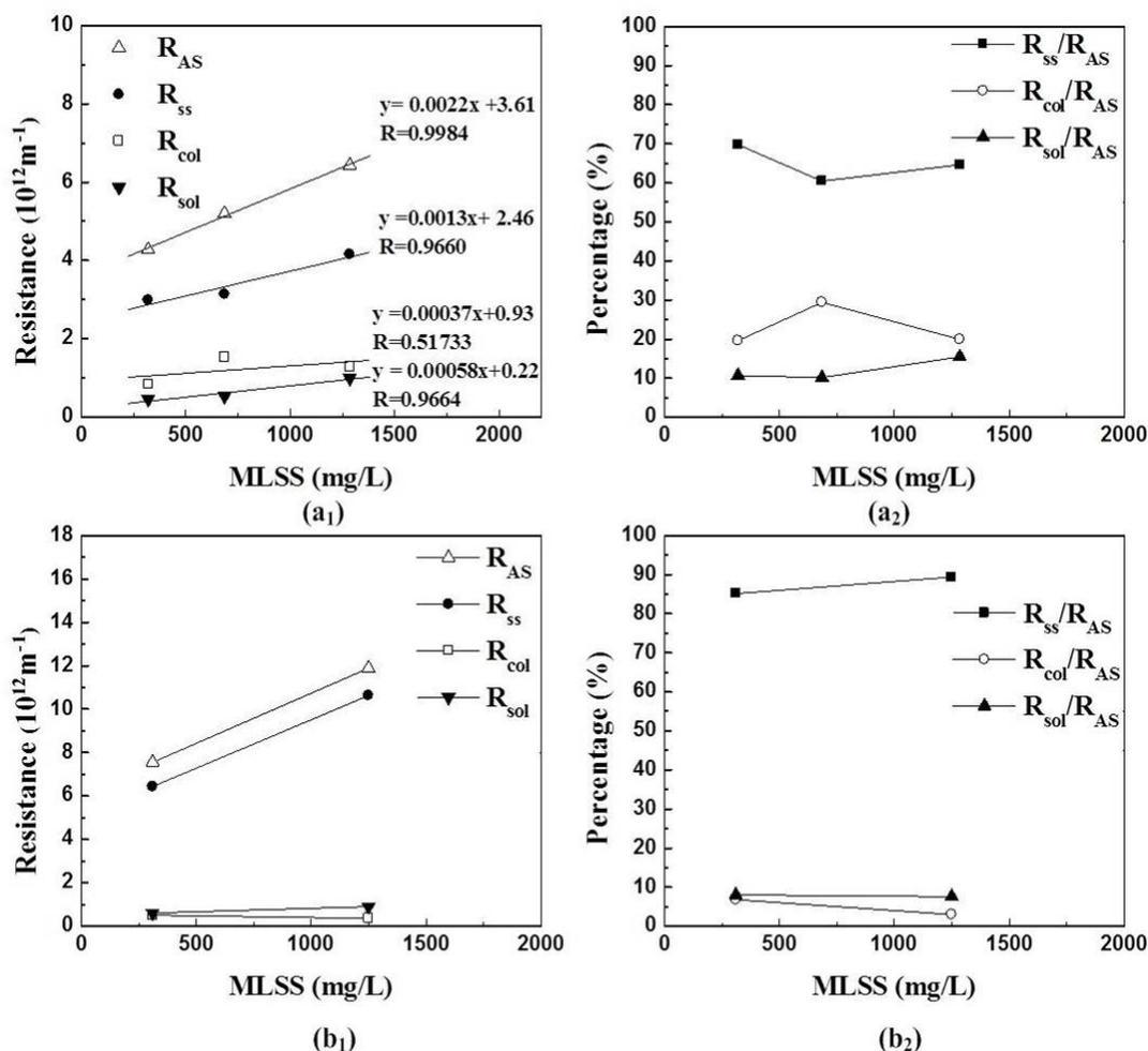
Fig. 3 Resistances of different sludge fractions according to MLSS concentration (a<sub>1</sub>), (a<sub>2</sub>) MBR; (b<sub>1</sub>), (b<sub>2</sub>) SBR (TMP = 1 bar, CFV = 0.438 m/s)
