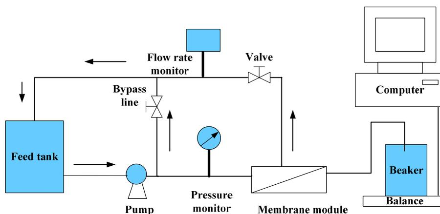
Fig. 1 Schematic diagram of crossflow membrane unit
