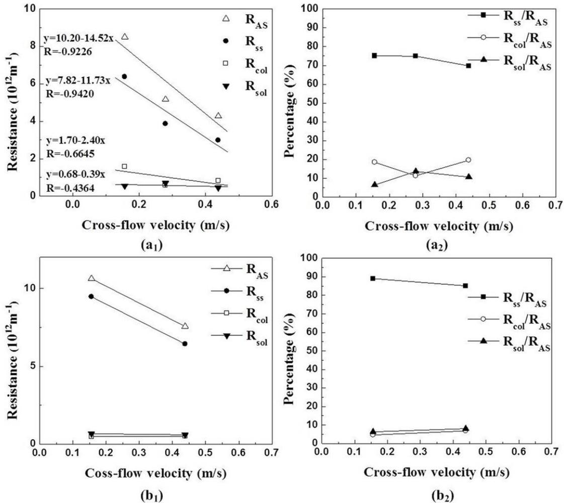
Fig. 5 Resistances of different sludge fractions according to cross-flow velocity (a<sub>1</sub>), (a<sub>2</sub>) MBR; (b<sub>1</sub>), (b<sub>2</sub>) SBR (MLSS = 320 mg/L, TMP = 1 bar)
