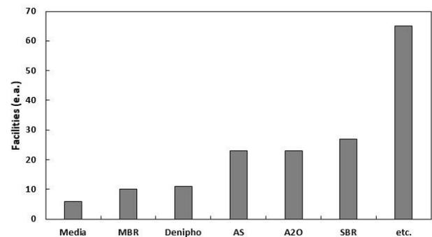
Fig. 8 Number of WWTP process in the Nakdong river basin (MBR: membrane bioreactor, AS: activated sludge, A2O: anaerobic/anoxic/oxic, SBR: sequencing batch reactor)
