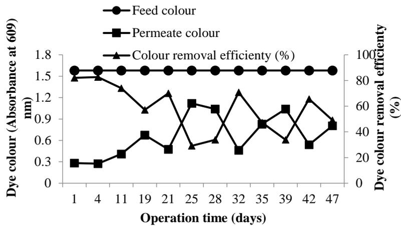
Fig. 3 Colour removal efficiency during SMBR experiment
