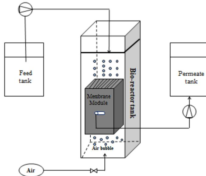
Fig. 1 Schematic representation of laboratory Submerged Membrane Bioreactor (SMBR) (⊗) Influent pump, (⊗) Air flow meter, (⊗) Effluent (permeate) pump
