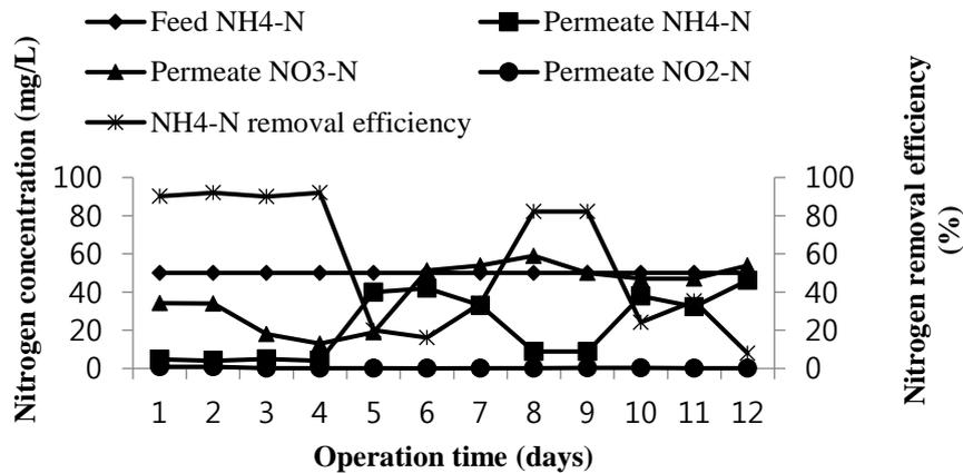
Fig. 4 Nitrogen removal efficiency during SMBR experiment
