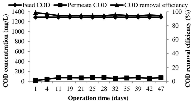
Fig. 2 COD removal efficiency during SMBR experiment
