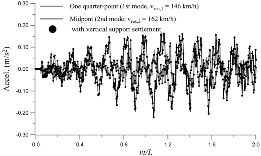
Fig. 5 Time history of acceleration of the suspended beam
