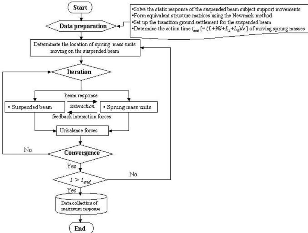
Fig. 3 Flow chart of incremental-iterative procedure
