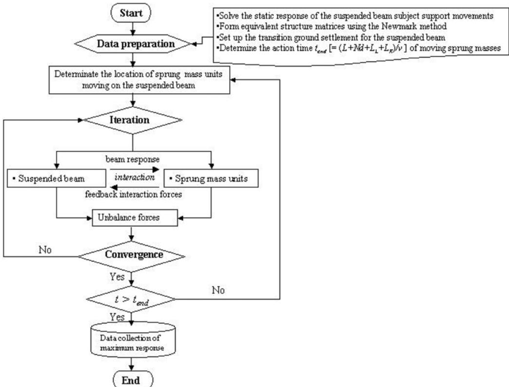
Fig. 3 Flow chart of incremental-iterative procedure
