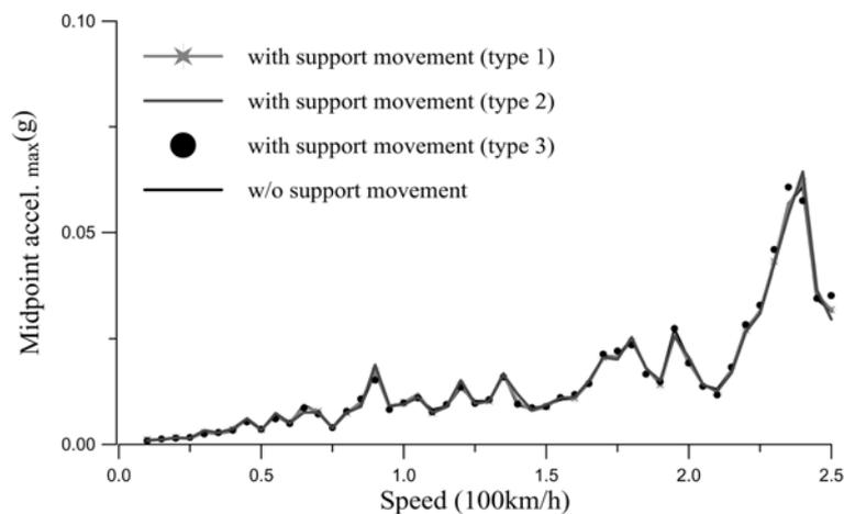
Fig. 8 Effect of support movements on beam response
