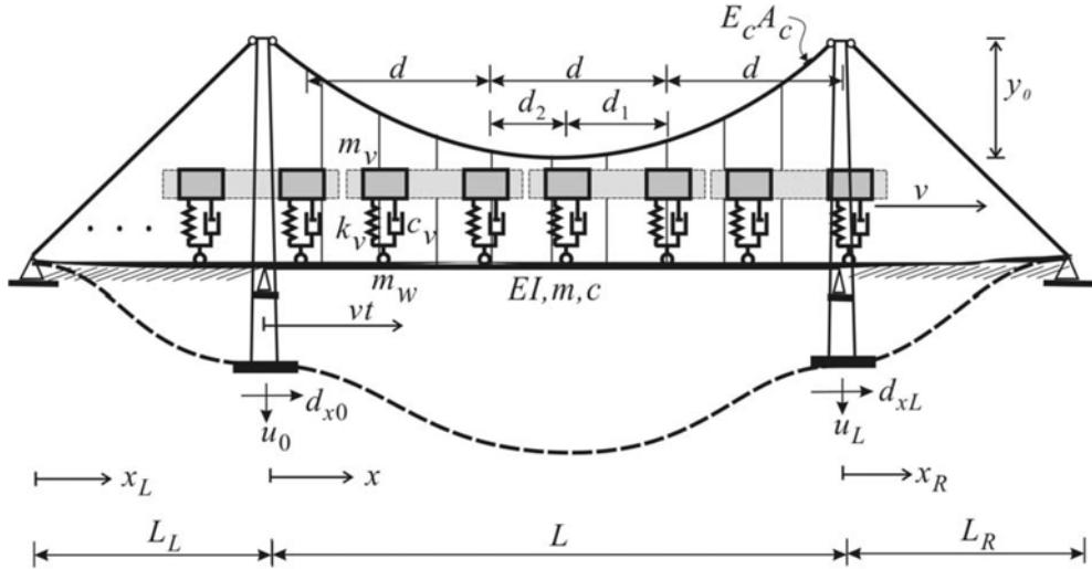
Fig. 2 A series of sprung masses cross a suspended beam with support movements
