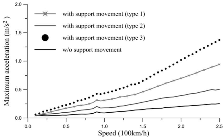
Fig. 7 Effect of support movements on  $a_{v,max} - v$  plots
