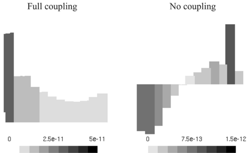
Fig. 11 Water tangential Darcian velocity profile inside the crack in m/s
