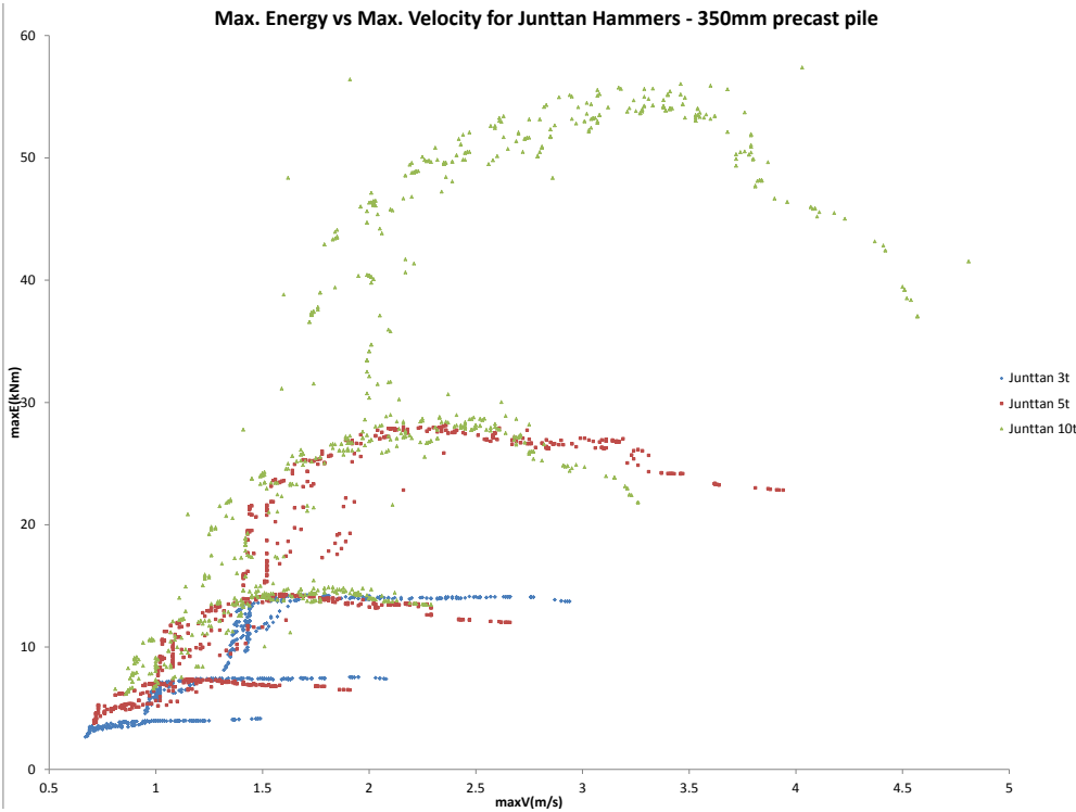
Fig. 6 Maximum energy versus velocity for Junttan hammer - concrete pile
