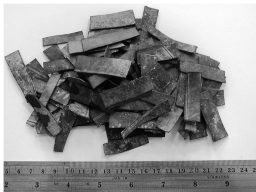
Fig. 2 A view of shredded tire rubbers used in this study (the scale of ruler is cm)
