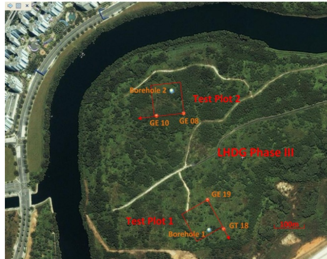
Fig. 2 Location of the test plots for geophysical investigation
