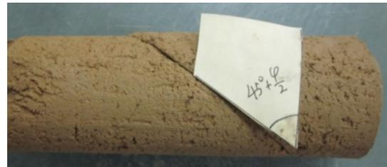
(b) Specimen in PTRD test
