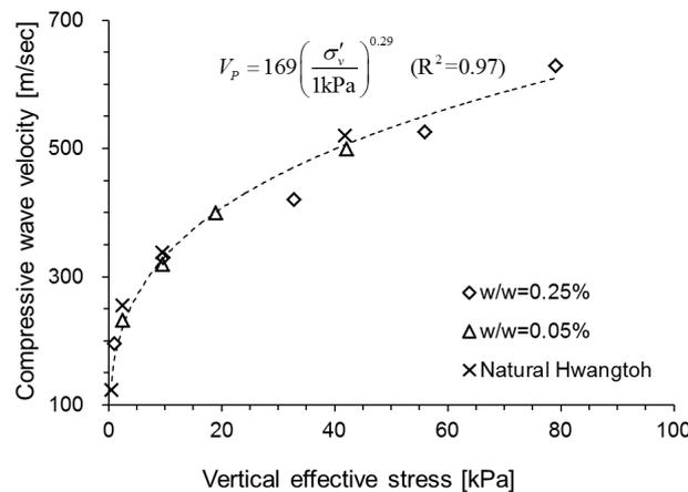
Fig. 7 Compressive wave velocity of  $\beta$ -1,3/1,6-glucan (BG) content treated Korean residual soil with vertical effective stress
