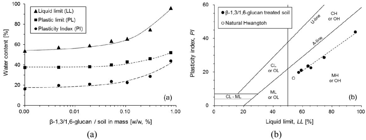
Fig. 3 Atterberg limits of  $\beta$ -1,3/1,6-glucan (BG) treated Korean residual soil: (a)  $LL$ ,  $PL$ , and  $PI$ ; (b) Plasticity chart
