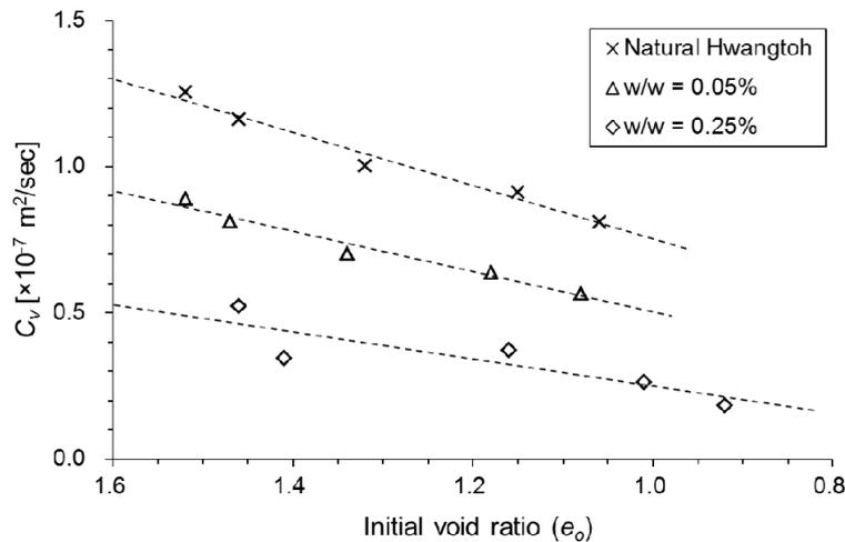
Fig. 4 Coefficient of consolidation ( $C_v$ ) of beta-1,3/1,6-glucan treated Korean residual soil
