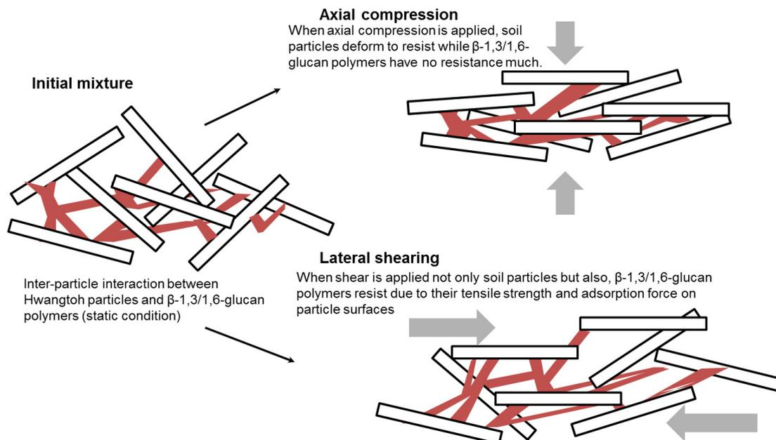
Fig. 8 Schematic model of the inter-particle behavior of  $\beta$ -1,3/1,6-glucan (BG) treated Korean residual soil
