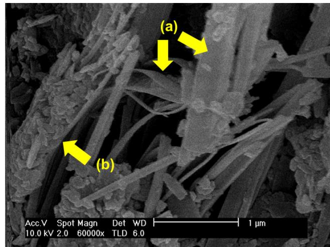
Fig. 2 SEM image of  $\beta$ -1,3/1,6-glucan (BG) treated Korean residual soil ( $w/w = 0.05\%$ ): (a) BG fibers with sparse soil particles attached; (b) Matrix of Korean residual soil particles and BG fibers
