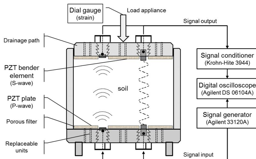
Fig. 1 Schematic diagram of instrumented consolidation testing device
