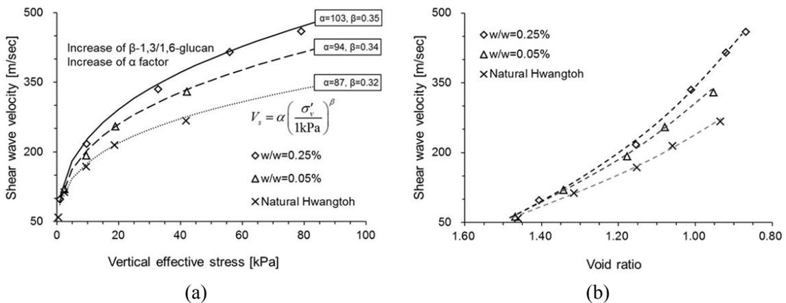
Fig. 6 Shear wave velocity of  $\beta$ -1,3/1,6-glucan (BG) content treated Korean residual soil: (a) with vertical effective stress; and (b) with void ratio
