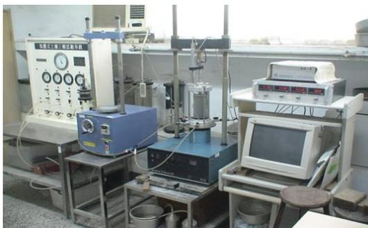
Fig. 4 Static triaxial test
