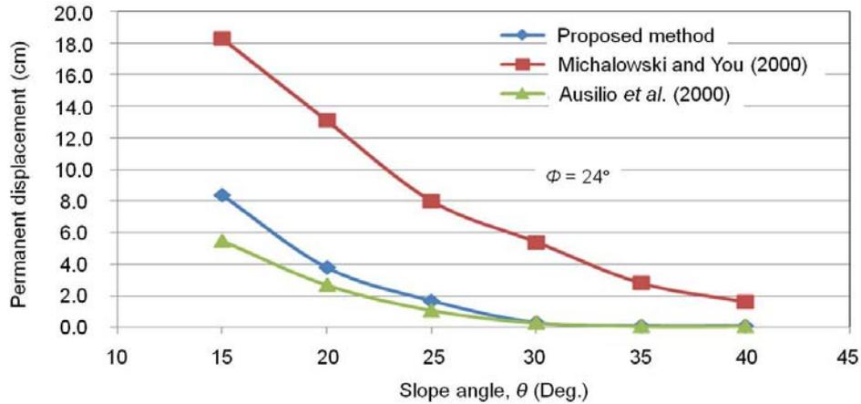
Fig. 18 Comparison of the displacements for the case where  $H = 5$  m,  $\Sigma T = 90$  kN/m,  $\phi = 24^\circ$
