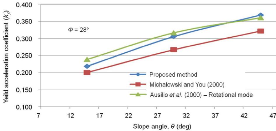
Fig. 15 Comparison of the  $k_y$  values obtained from different methods for various angles of slope at  $\phi = 28^\circ$
