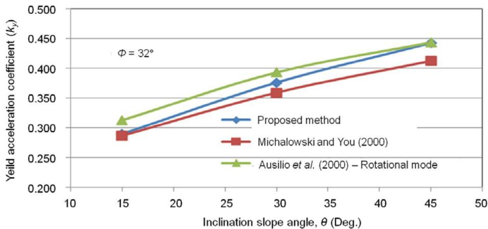
Fig. 16 Comparison of the  $k_y$  values obtained from different methods for various angles of slope at  $\phi = 32^\circ$
