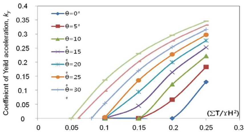
Fig. 20 Design chart for  $k_y$  ( $\phi = 25^\circ$ )
