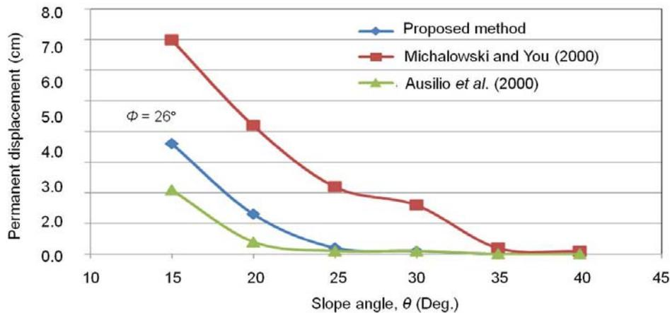
Fig. 19 Comparison of the displacements for the case where  $H = 5$  m,  $\Sigma T = 90$  kN/m,  $\phi = 26^\circ$
