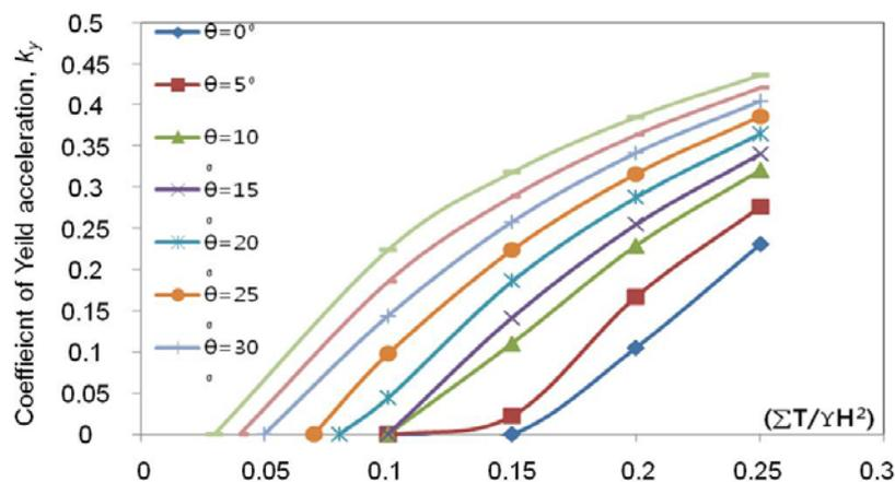
Fig. 21 Design chart for  $k_y$  ( $\phi = 30^\circ$ )
