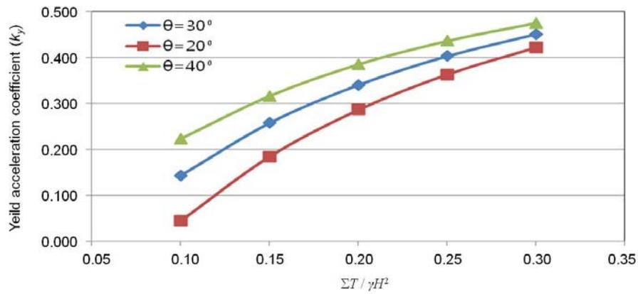
Fig. 9 Variations of the coefficient of yield acceleration against  $\Sigma T / \gamma H^2$  ( $\phi = 30^\circ$ )
