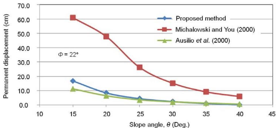
Fig. 17 Comparison of the displacements for the case where  $H = 5\text{ m}$ ,  $\Sigma T = 90\text{ kN/m}$ ,  $\phi = 22^\circ$
