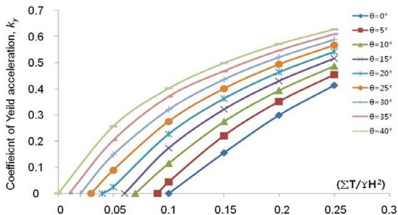
Fig. 23 Design chart for  $k_y$  ( $\phi = 45^\circ$ )
