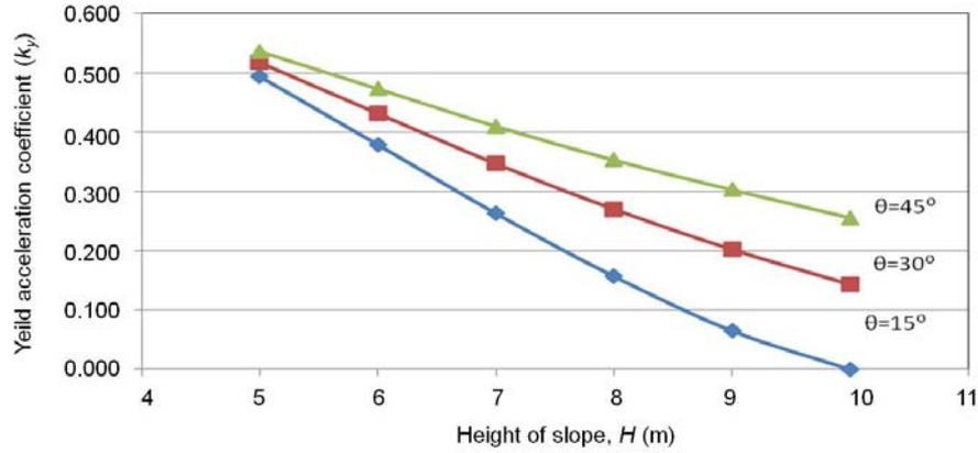
Fig. 8 Variations of the coefficient of yield acceleration against the height of the slope ( $\Sigma T = 180$  kN/m,  $\phi = 30^\circ$ )
