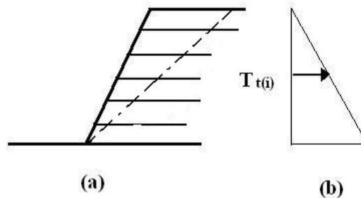
Fig. 1 (a) Reinforced slope and failure wedge; (b) force distribution in reinforcements along the height
