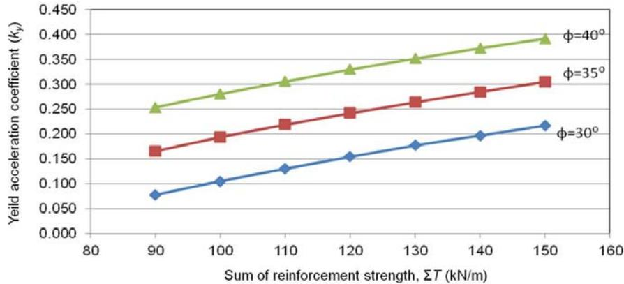
Fig. 6 Variations of the coefficient of yield acceleration against the sum of reinforcing forces ( $H = 8$  m,  $\theta = 30^\circ$ )
