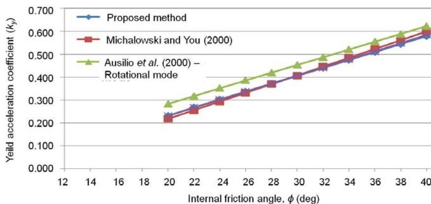
Fig. 12 Comparison of the critical accelerations for the case where  $H = 5$  m,  $\theta = 15^\circ$ ,  $\Sigma T = 135$  kN/m,  $\gamma = 18$  kN/m<sup>3</sup>
