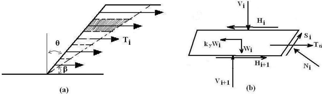
Fig. 2 (a) Divided slope into horizontal slices; (b) a separated horizontal slice and the forces acting on it
