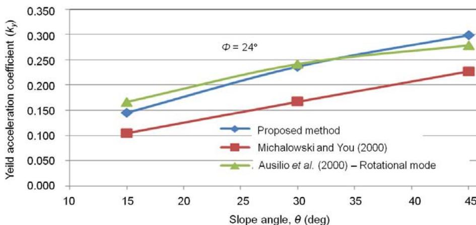
Fig. 14 Comparison of the  $k_y$  values obtained from different methods for various angles of slope at  $\phi = 24^\circ$
