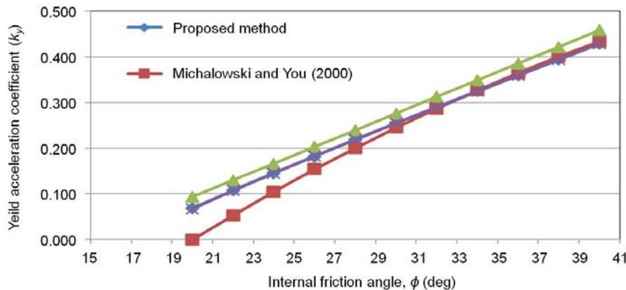
Fig. 11 Comparison of the critical accelerations for the case where  $H = 5$  m,  $\theta = 15^\circ$ ,  $\Sigma T = 90$  kN/m,  $\gamma = 18$  kN/m<sup>3</sup>
