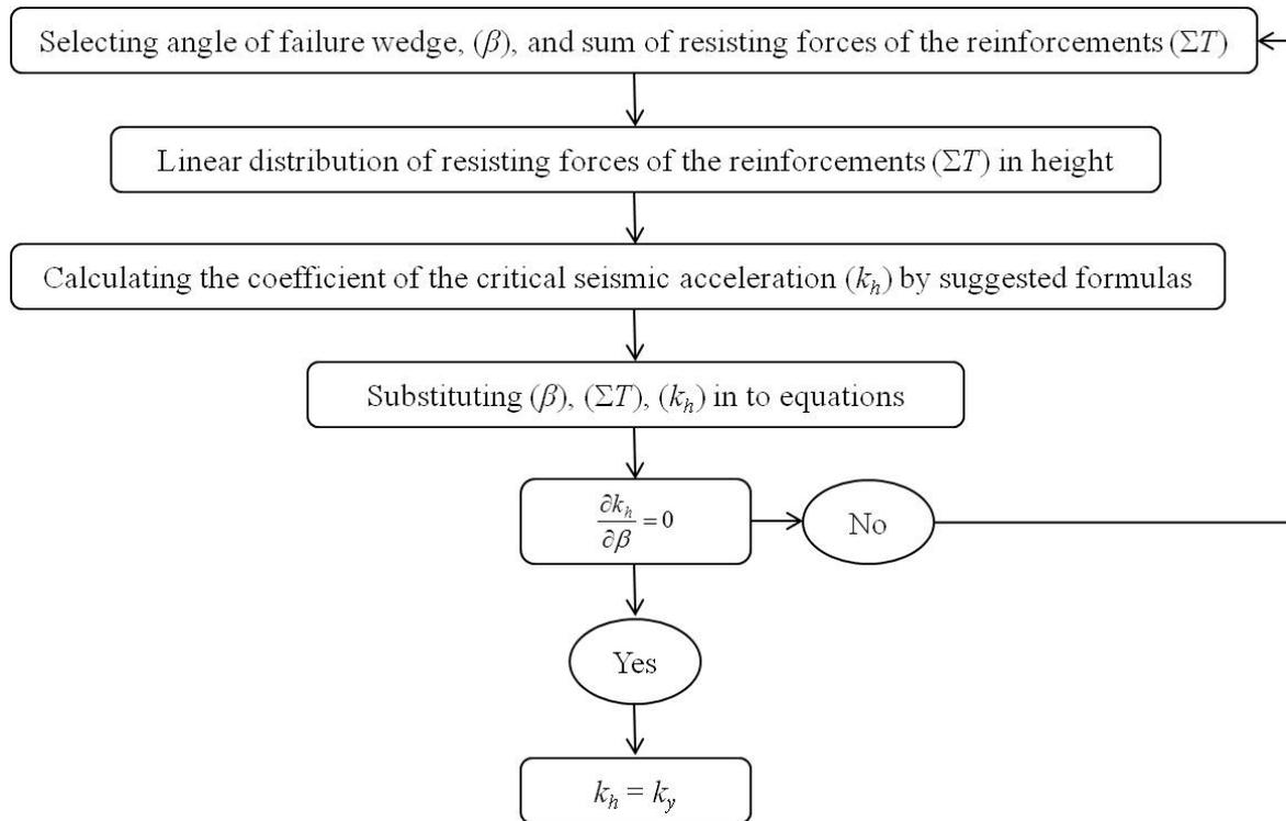
Fig. 3 Algorithm used to determine the yield acceleration
