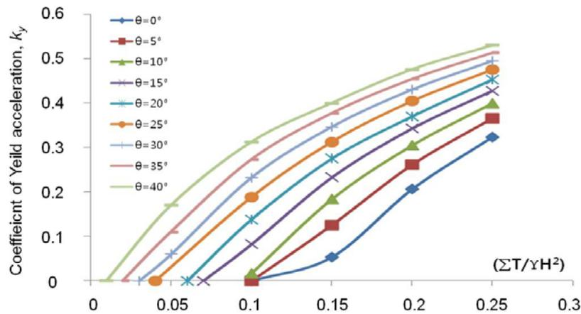
Fig. 22 Design chart for  $k_y$  ( $\phi = 40^\circ$ )
