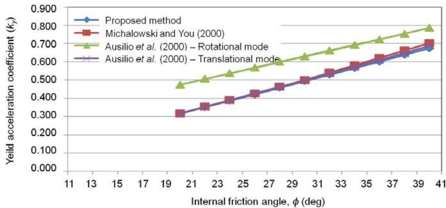
Fig. 13 Comparison of the critical accelerations for the case where  $H = 5$  m,  $\theta = 15^\circ$ ,  $\Sigma T = 180$  kN/m,  $\gamma = 18$  kN/m<sup>3</sup>
