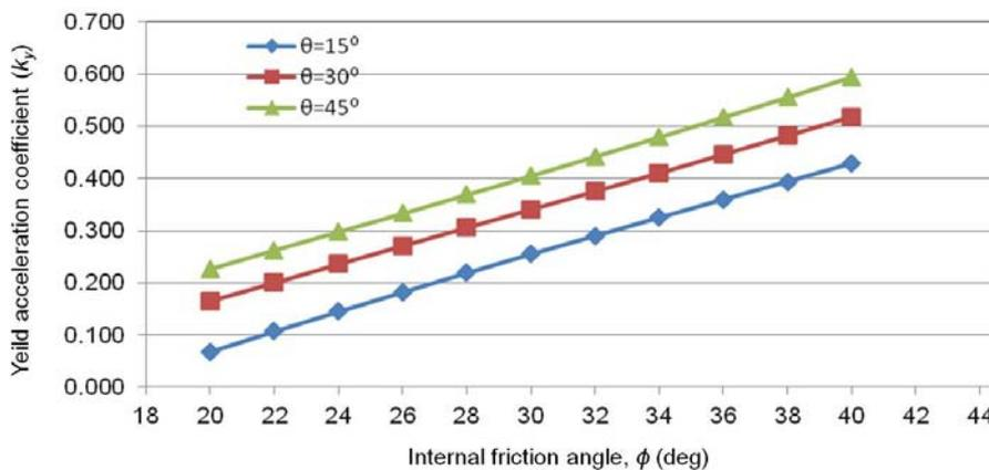
Fig. 5 Variations of the coefficient of yield acceleration against the internal friction angle of the soil ( $H = 5 \text{ m}, \Sigma T = 90 \text{ kN/m}$ )
