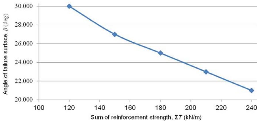
Fig. 4 Variations in the angle of failure wedge against  $\Sigma T$  ( $\theta = 40^\circ, \phi = 20^\circ$ )
