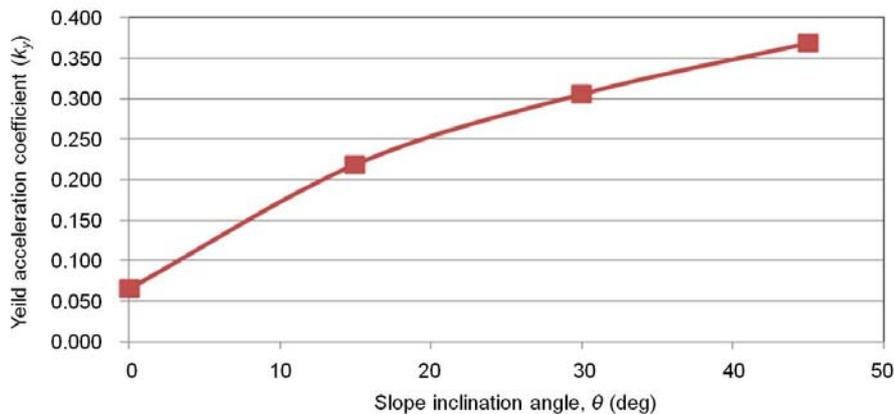
Fig. 7 Variations of the coefficient of yield acceleration against the slope inclination angle ( $H = 5$  m,  $\phi = 28^\circ$ ,  $\Sigma T = 90$  kN/m)
