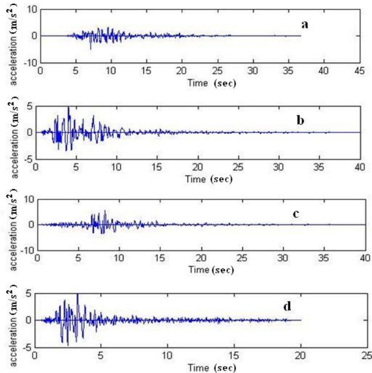
Fig. 10 Records of the used earthquakes (a) Kobe; (b) Loma Prieta; (c) Northridge; (d) Palm Spring
