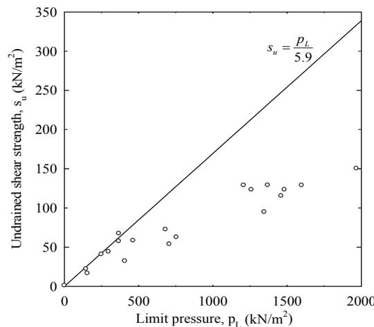
(a) Correlation between undrained shear strength ( $s_u$ ) and limit pressure ( $p_L$ )
