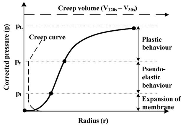
Fig. 7 Typical result for the LLT pressuremeter test
