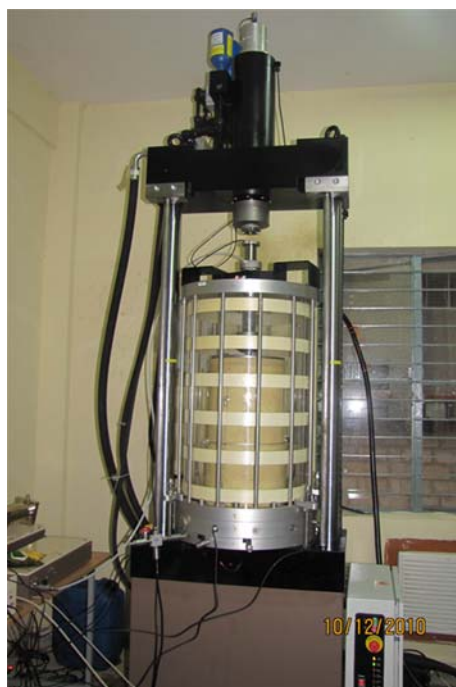
Fig. 1 Cyclic triaxial set up in the Geotechnical Engineering Laboratory of Indian Institute of Science
