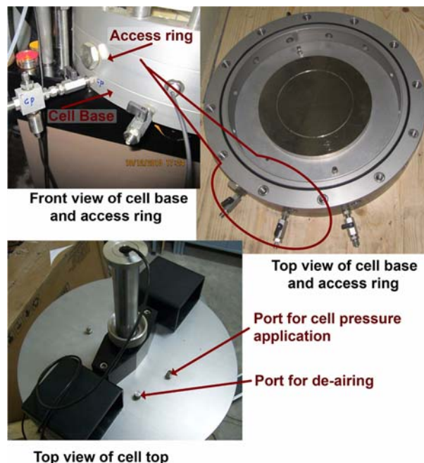
Fig. 2 Parts of the triaxial cell
