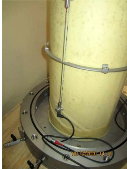
Fig. 3 Triaxial sample of 300 mm diameter and 600 mm height with LVDT's for local axial and radial strain measurements
