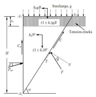
Fig. 1 Forces acting on a trial failure wedge consisting of c- $\phi$  soil backfill with tension cracks behind a rigid retaining wall in active state
