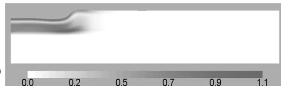
Fig. 14 Variation in viscoplastic shear strain during construction (after 215 days)
